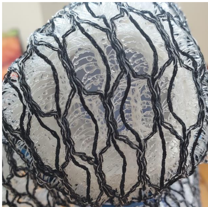
Figure 10. PBL Fog Unit Prototype 3: close up of water deposition on net
