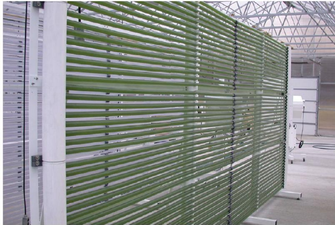
Figure 8: Tubular Photobioreactor (Greenwell et al., 2010)
