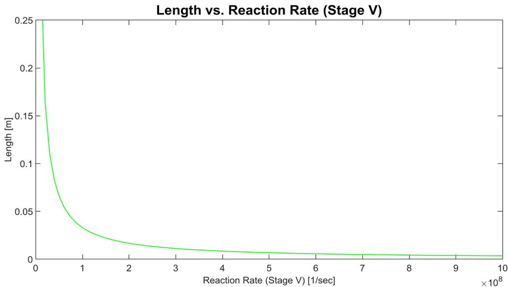
**Figure 17.** The length of the catalyst bed varies greatly with the associated reaction rate of the catalyst and hydrogen peroxide.
