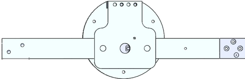
**Figure 22.** A top view of the torsional thrust stand.
