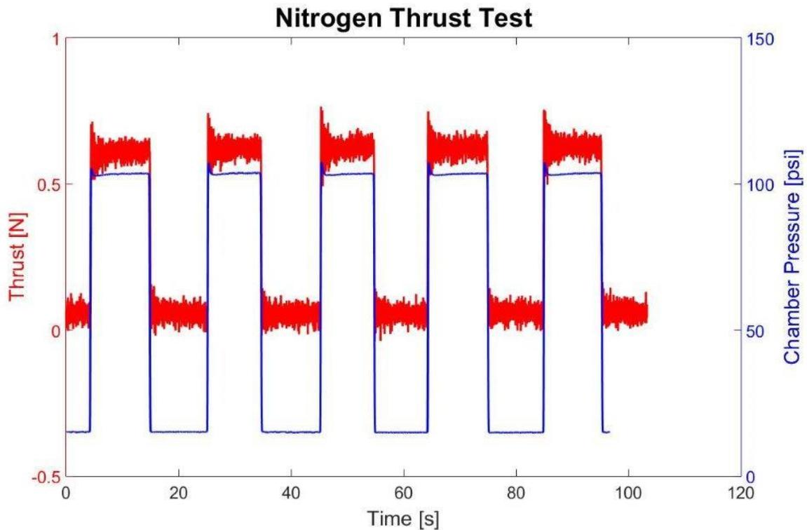
**Figure 39.** Test firing began with nitrogen gas to validate the system. A thrust of .6 N and chamber pressure of 100 psi was achieved, as anticipated.
