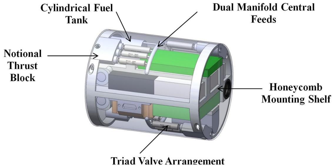
**Figure 14.** The objective propulsion system was designed to meet the volume constraints of the CanSat concept.
