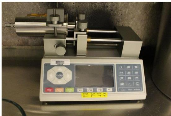
**Figure 30.** A Nexus 6000 syringe pump was used to contain and pressurize the propellant.
