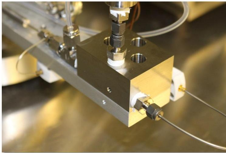
**Figure 29.** Installation of the thrust block onto the thrust stand proved easy and robust.
