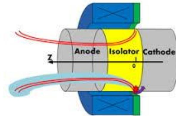
**Figure 8.** A vacuum arc thruster operates by ejecting cathode material.
