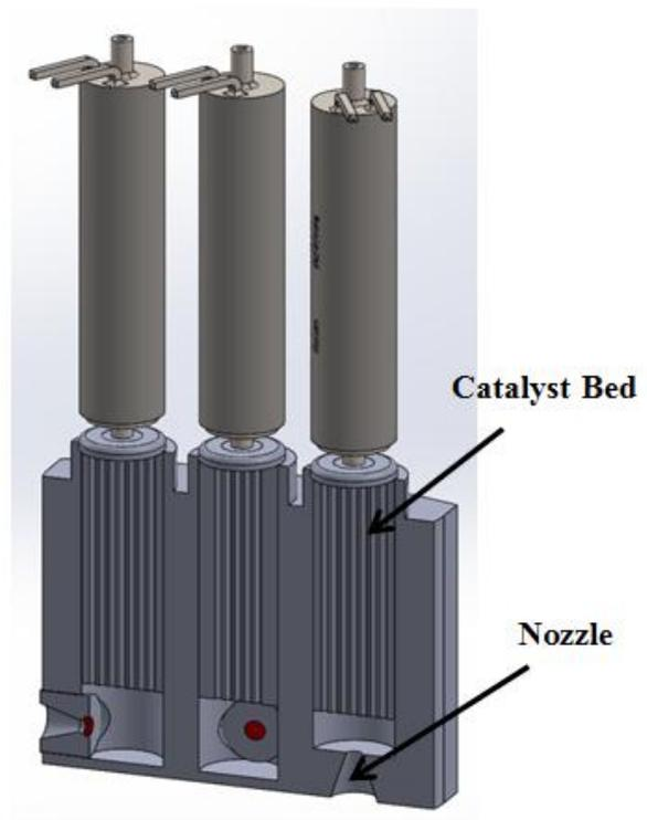
**Figure 15.** A design concept for the flight system centers on a triad design.
