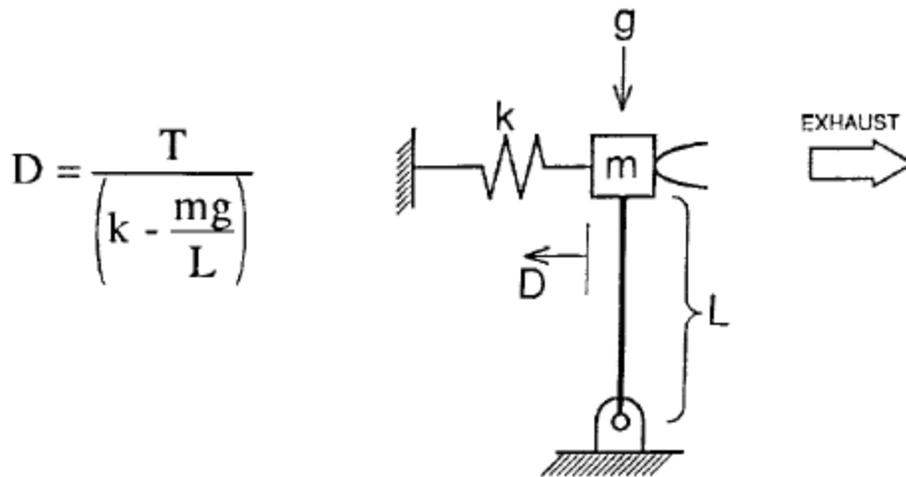
**Figure 20.** A schematic illustrates the functionality of an inverted pendulum thrust stand [Haag, 1989].
