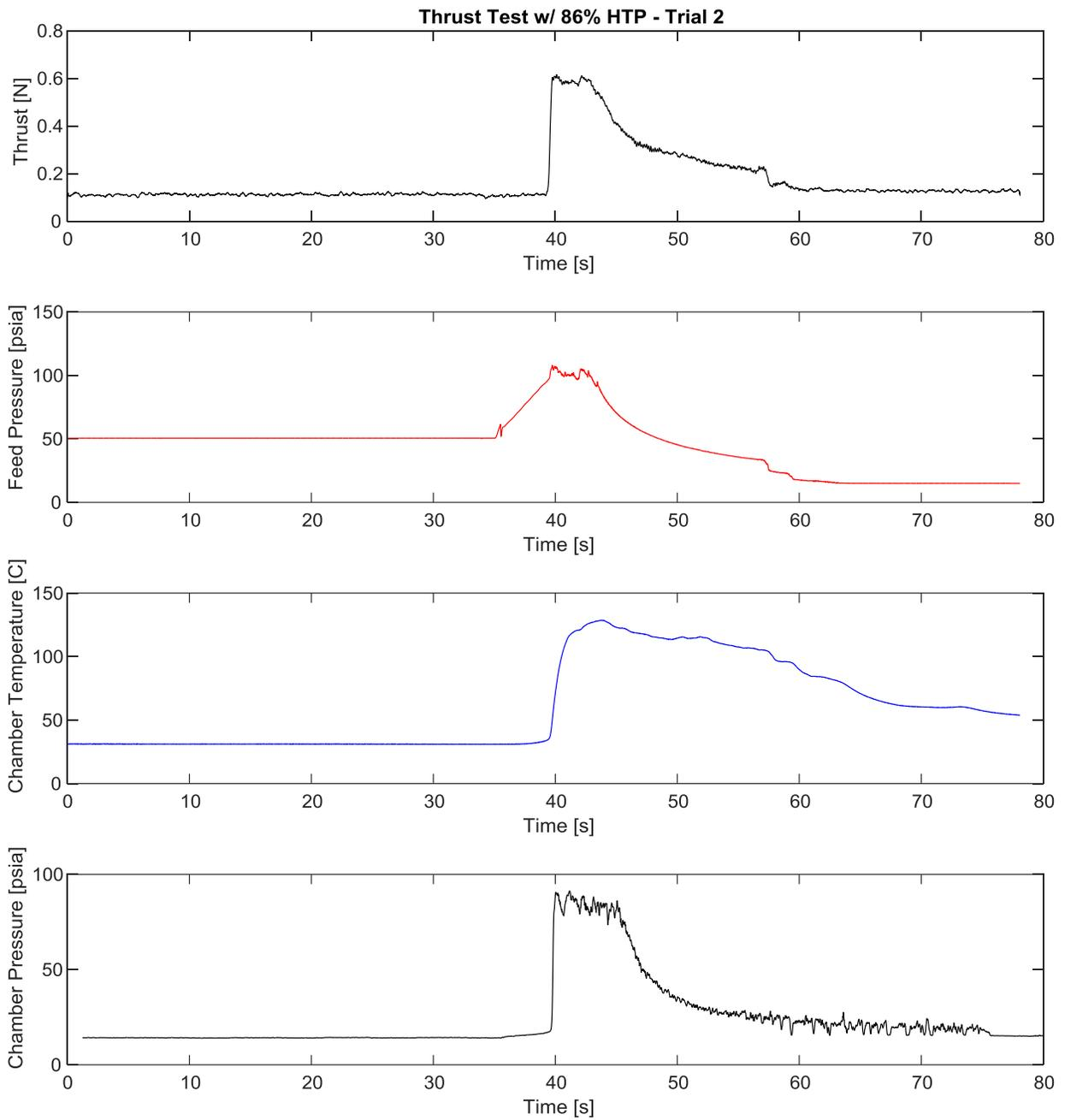
**Figure 42.** The second test fire began achieved similar results as Trial 1, with .5 N of thrust, a feed pressure that quickly climbed to 100 psia, a chamber temperature of 135 C, and a chamber pressure around 90 psia.
