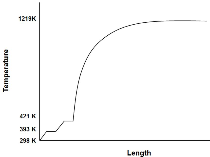
**Figure 16.** The decomposition process can be divided into five distinct sub-regions, based on temperature, for the purpose of deriving an analytical model based on energy conservation.
