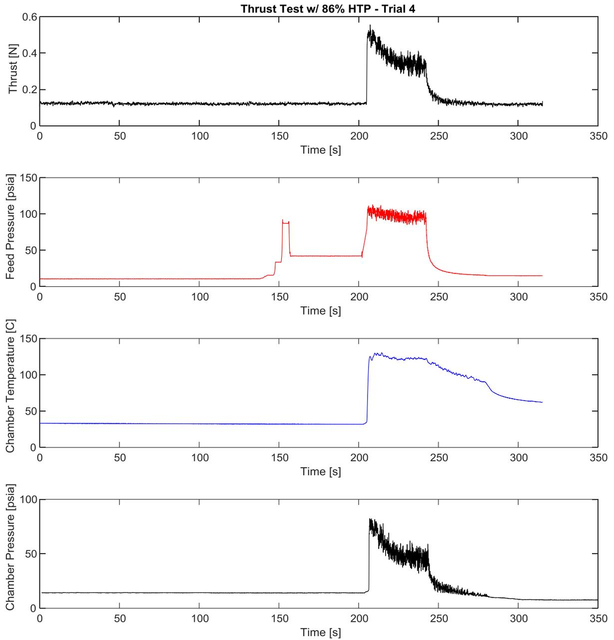
**Figure 44.** A final attempt at a long duration test fire resulted in a spike of expected performance, which quickly fell to a steady state at half the thrust and chamber pressure previously achieved.
