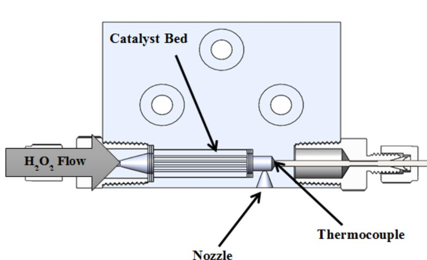
**Figure 19.** The experimental thruster block attempted to recreate an arrangement similar to that expected in the objective design.
