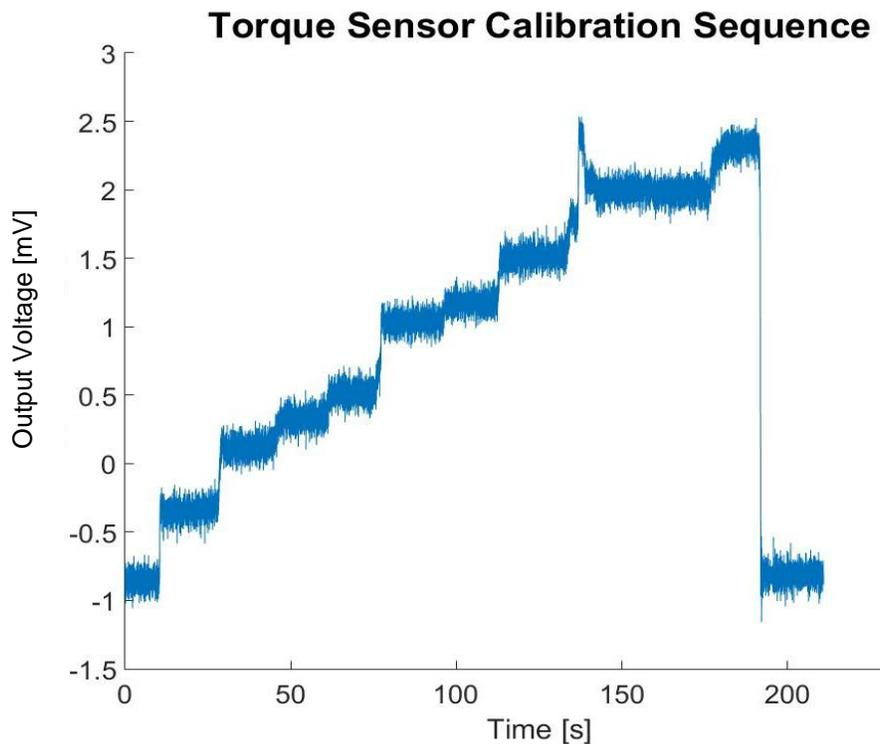
**Figure 36.** The calibration sequence for the torque sensor required several seconds of voltage data be collected at a recorded force applied.
