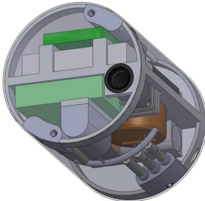
**Figure 13.** The concept of the CanSat was developed to provide volume constraints for a proposed picosatellite system. Propulsion system
