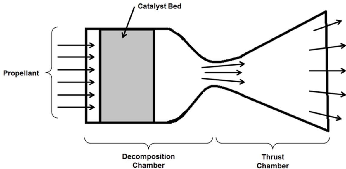
**Figure 5.** Monopropellant thrusters work through the expansion of gases created by the exothermic decomposition of propellant.
