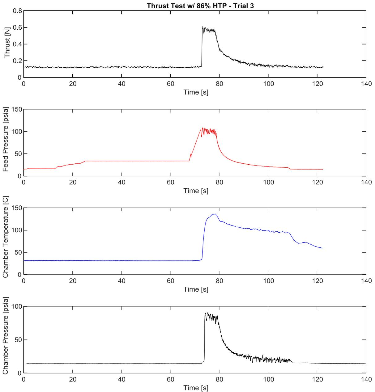
**Figure 43.** To begin Trial 3, the initial feed pressure was lowered to 30 psia, but quickly climbed to 100 psia once more. Similar results were obtained, but indications concerning the validity of the syringe pump as a pressurizing device arose.
