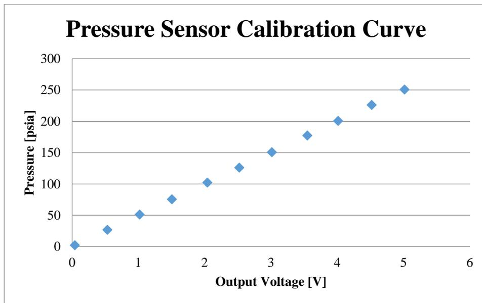
**Figure 38.** Manufacturer data was used to generate the calibration curve for the Setra pressure sensor.
