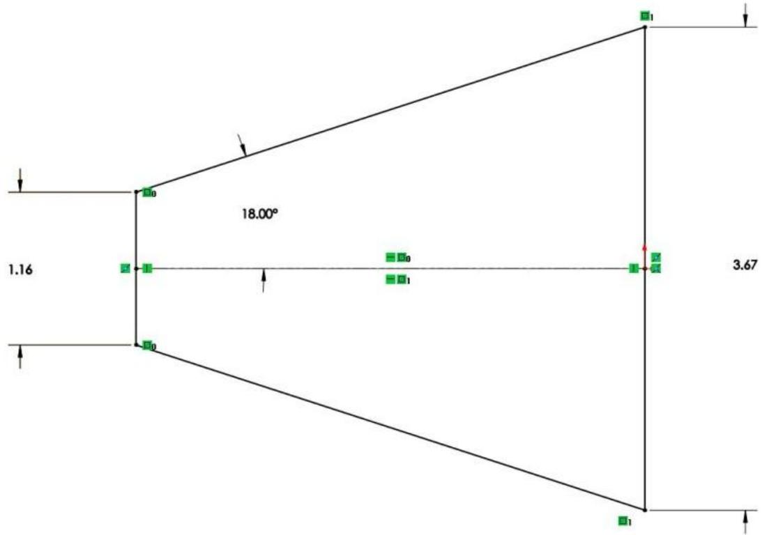
**Figure 18.** A conical nozzle was chosen to simplify the machining process.
