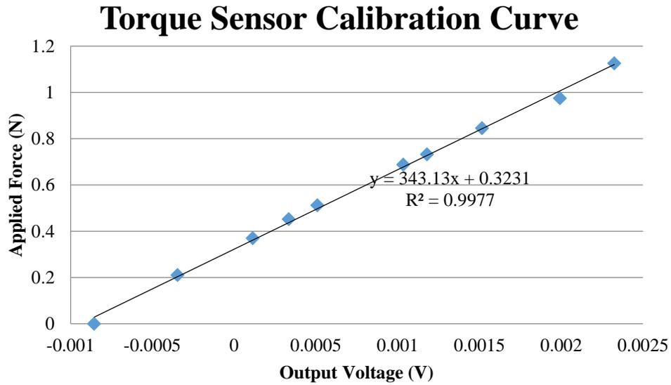
**Figure 37.** The values of applied force and output voltage of the torque sensor were correlated via a calibration curve.
