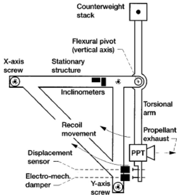
**Figure 21.** A schematic illustrates the functionality of a PPT torsional thrust stand [Haag, 1989].
