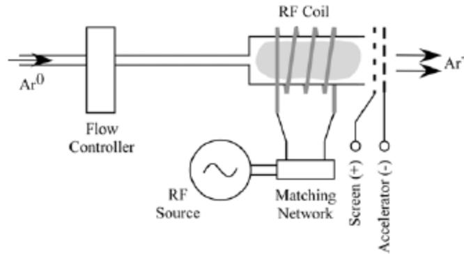
**Figure 9.** The thruster developed by Penn State uses micro-ion technology to generate low thrust.
