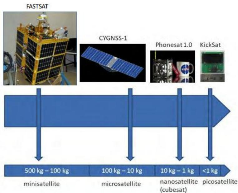
**Figure 3.** NASA has conducted work on classifying these small satellite categories [Frost et al, 2014].
