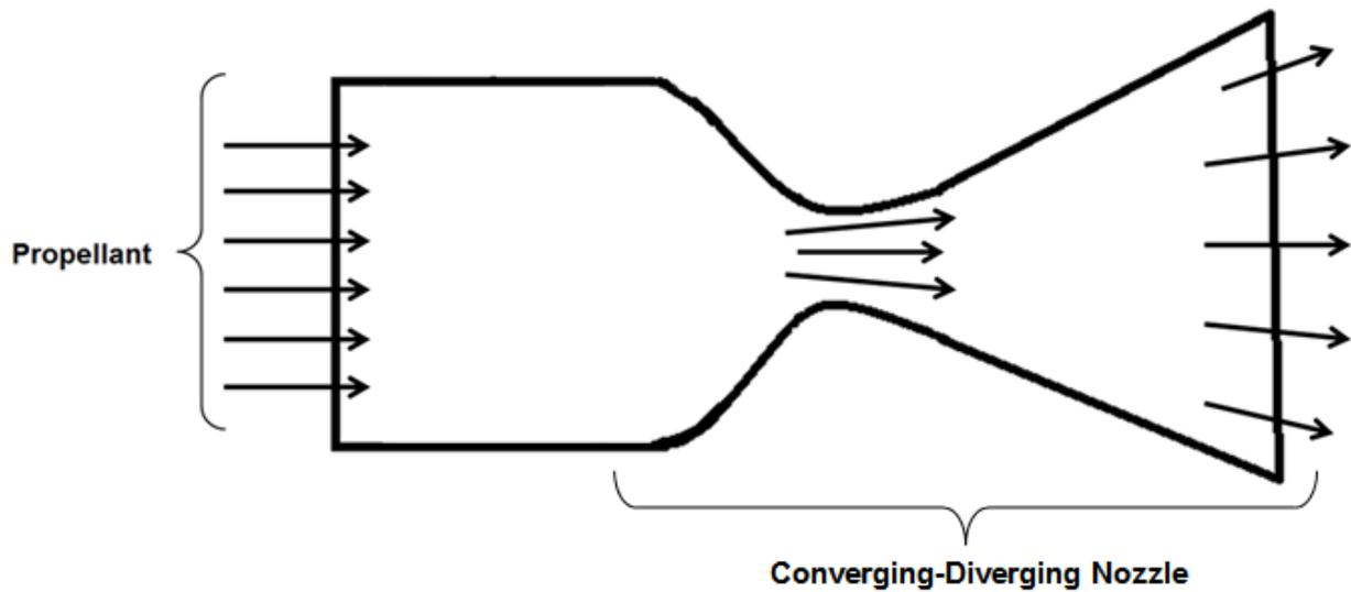
**Figure 6.** A cold gas thruster operates through expanding a gas from an area of high pressure to an area of low pressure via a converging diverging nozzle.
