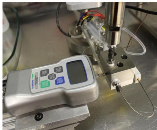
**Figure 35.** An accurate force gauge was used to provide a known force in order to calibrate the torque sensor.
