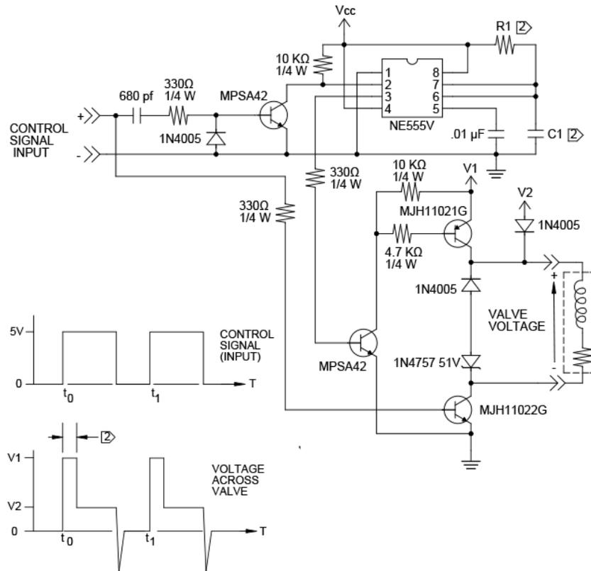
**Figure 32: Valve Driver Circuit Diagram**
