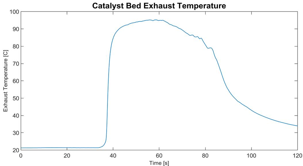
**Figure 40.** A test of the 1 cm long catalyst attempted to characterize percent of theoretical adiabatic decomposition temperature reached.
