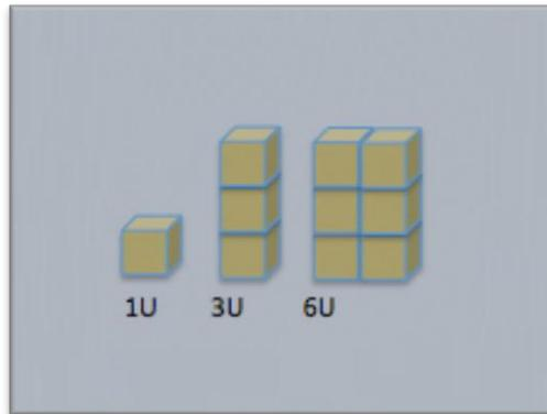
**Figure 4.** The standard frames for a CubeSat center on the compilation of single units (1U) [Mehrparvar, 2014]
