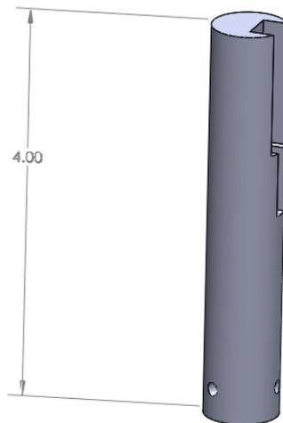
**Figure 27.** In addition to providing the center axis for the torque arm, a slot in the top of the shaft allows for tubing and wiring to be fed through the center. This attempts to negate irregularities in thrust measurement.
