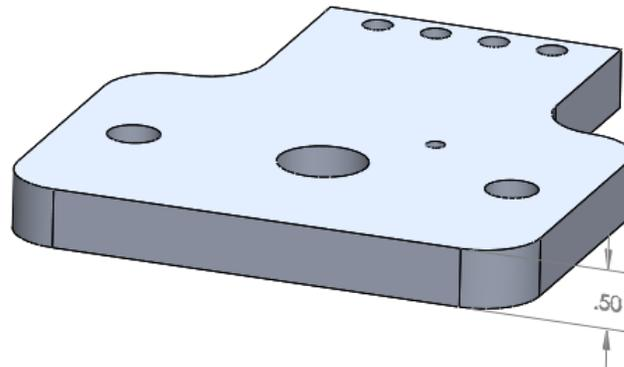
**Figure 26.** An isometric view of the top of the thrust stand. A bearing attaches to this piece, allowing for free rotation of the shaft
