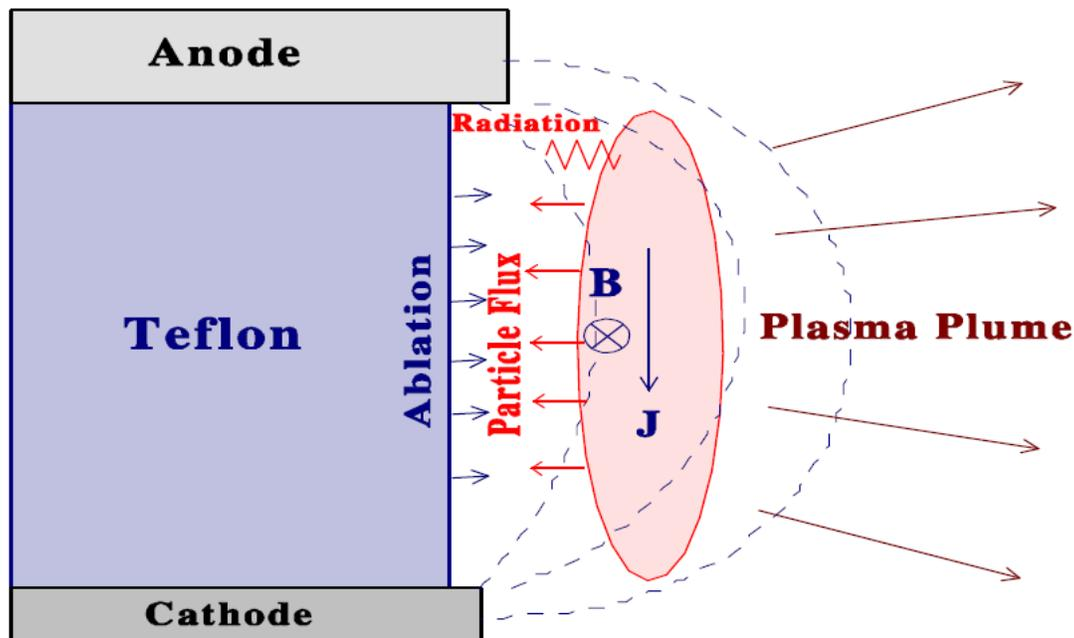
**Figure 7.** A pulsed plasma thruster ablates particles of Teflon between two electrodes [Spanjers, 2002].
