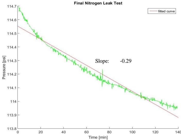
**Figure 34.** A test of the system with nitrogen gas indicated initial leaks in the system. Changes were made to provide a leak free system for hydrogen peroxide use.
