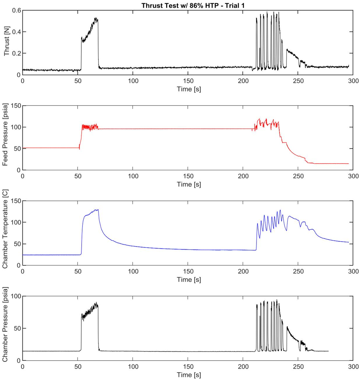
**Figure 41.** The first test fire consisted of two distinct sections. The valve was initially switched on at 50 seconds and performance increased as catalyst bed warmed up. The second phase was a series of manual pulses until the line was emptied. A thrust between .3 and .6 N was generated with a feed pressure of 100 psia, chamber temperature of 135 C, and chamber pressure approaching 100 psia.
