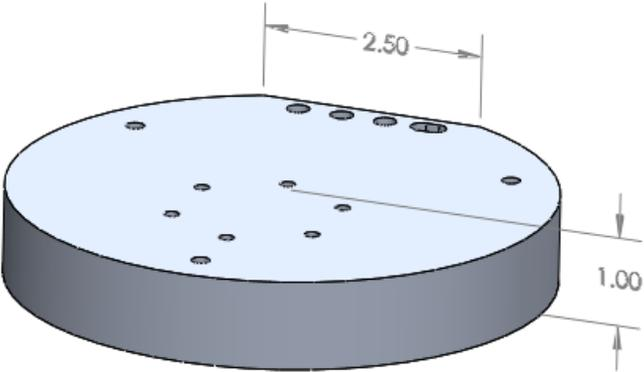
**Figure 24.** An isometric view of the thrust stand base.
