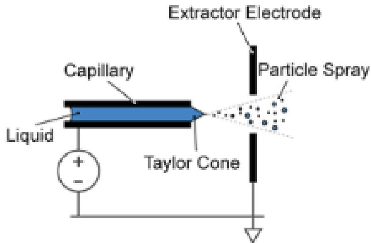
**Figure 10.** Electro spray thrusters operate by discharging ions in an electric field [Mueller et al, 2010].
