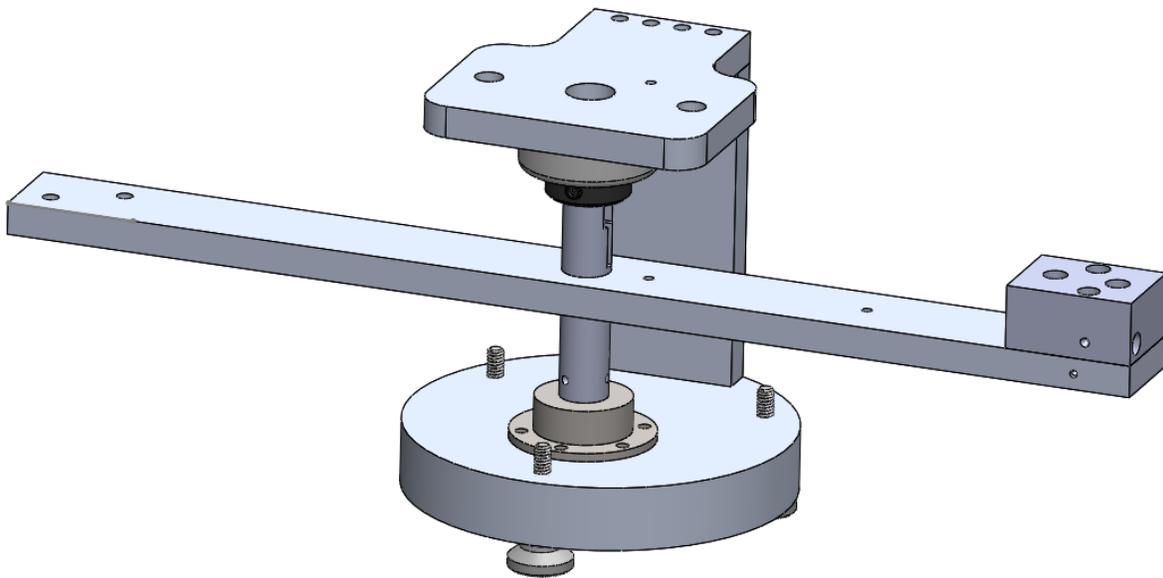
**Figure 23.** An isometric view of the thrust stand design.
