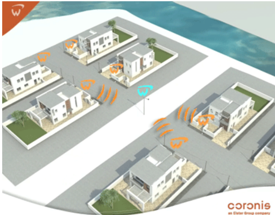
Figure 7: A pictorial representation of a communications network utilising a gateway (Coronis, n.d. )
