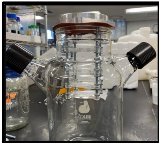
Figure 8: Final Iteration of Collection Vessel Top
