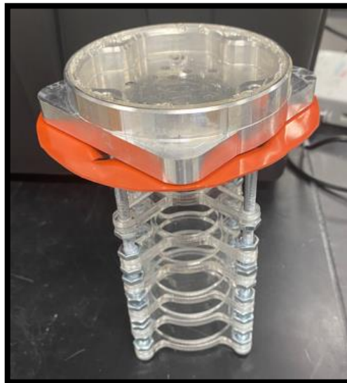
Figure 27: Vessel Collection Assembly
