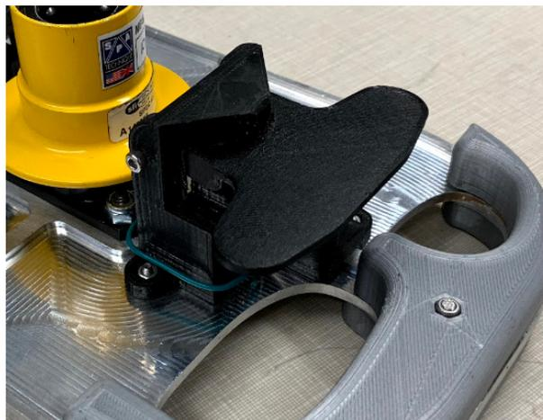
Figure 56: *3D Printed Paddle Shifter Assembly*
