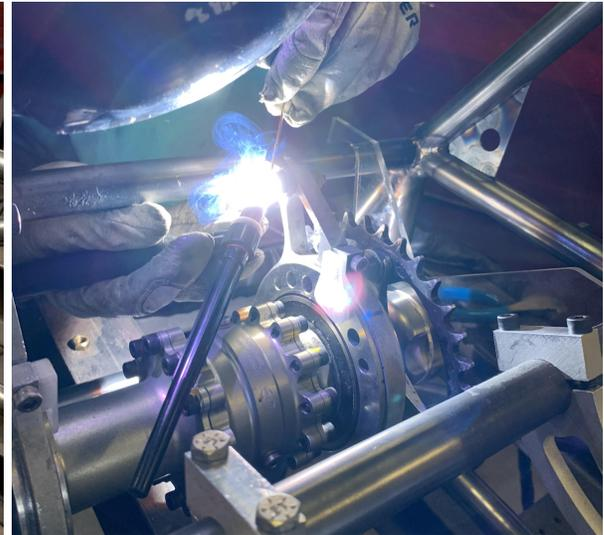
Figure 41: Differential tab welding
