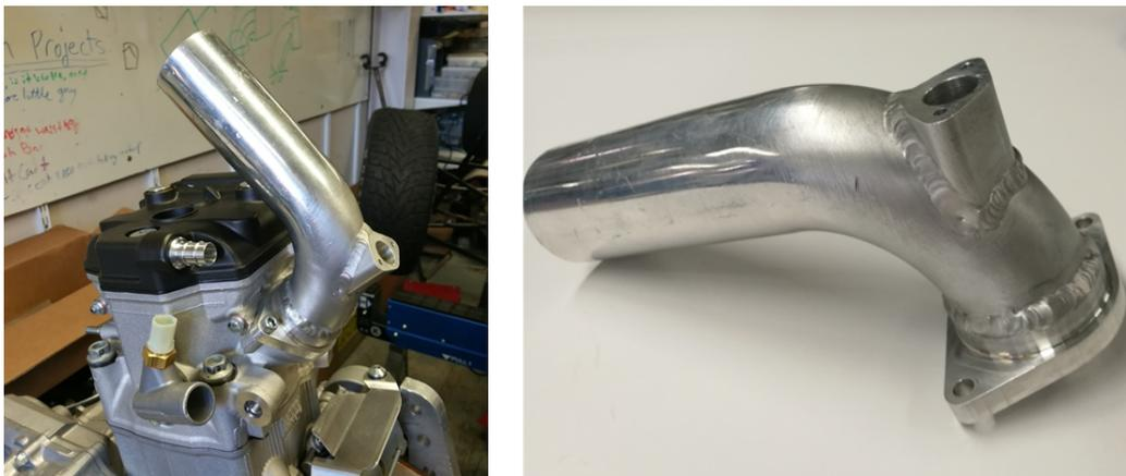
Figure 66: *Intake Flange and Injector Tube*
