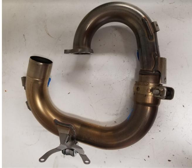
Figure 78: *Yamaha Exhaust Header Piping.*
