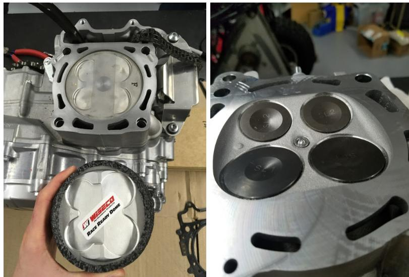
Figure 61: *Yamaha and Wiseco Pistons, & WR450F Pentroof*
