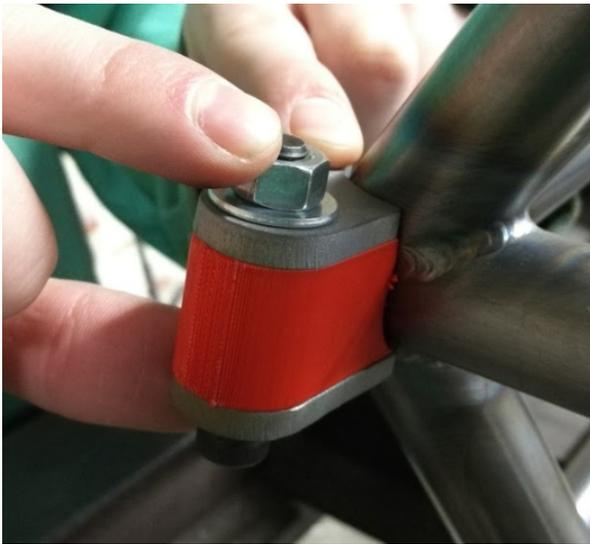
Figure 33: *Rear tab with 3D printed fixture.*
