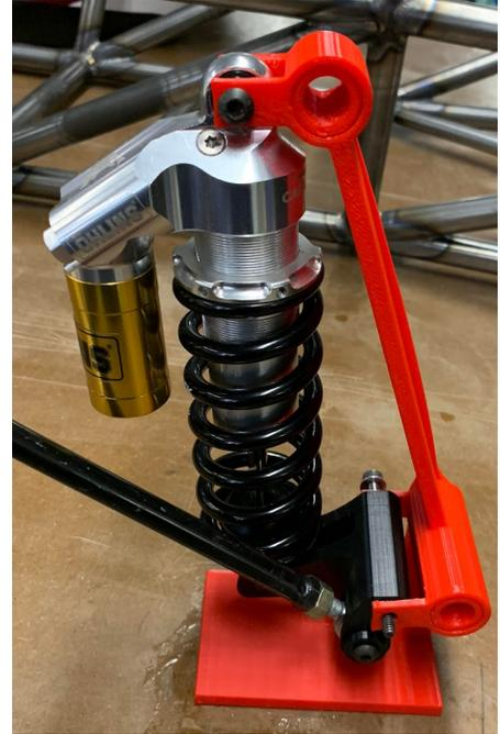
Figure 131: Rear suspension mockup
