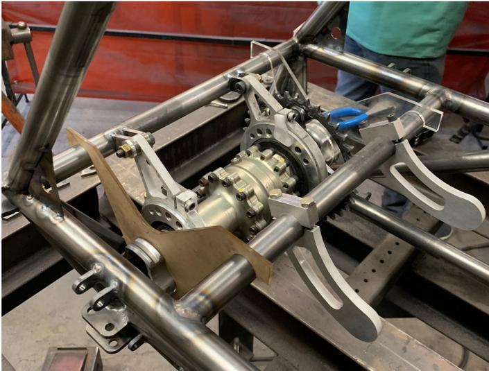
Figure 40: Differential mount tooling
