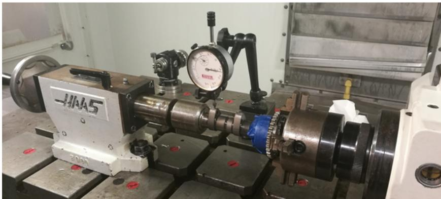
Figure 81: *Camshaft Lift and Duration Measurement with CNC Mill and Dial Indicator.*
