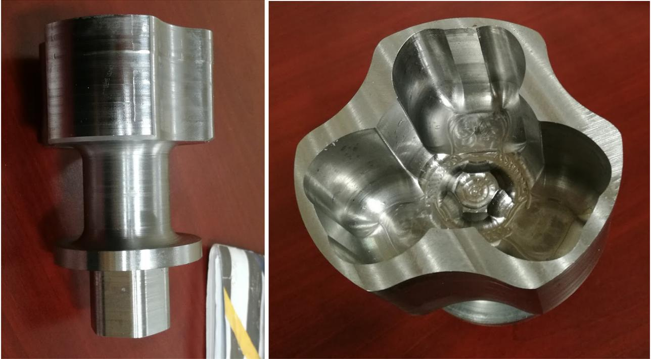
Figures 48: *Machined Axle Housings*
