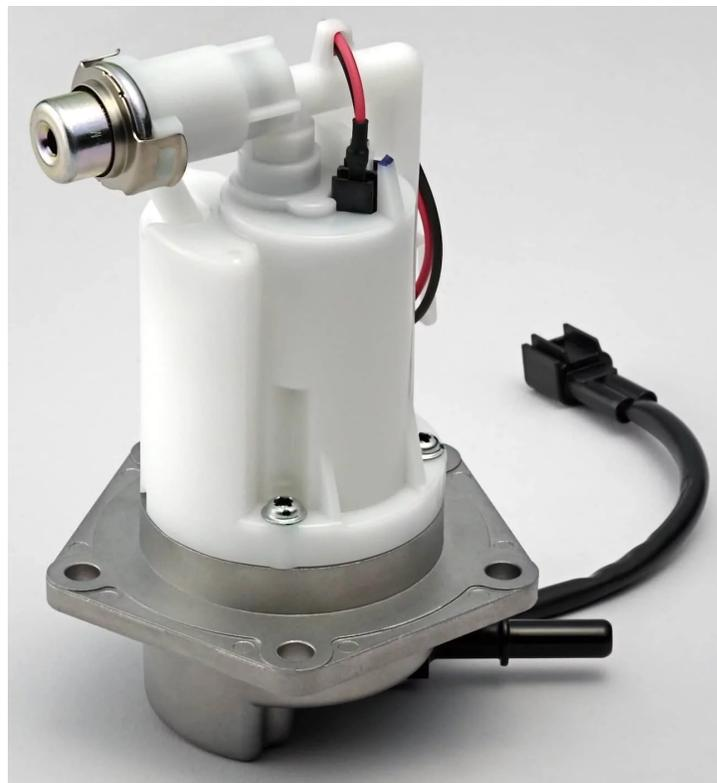
Figure 72: Suzuki RMZ450 Fuel Sending Unit [23]
