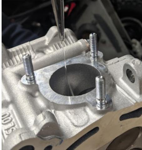
Figure 79: *Port Volume Measurement*
