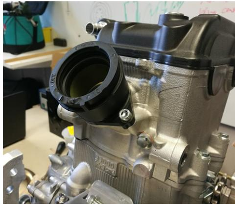
Figure 65: *Factory Yamaha Intake Boot*
