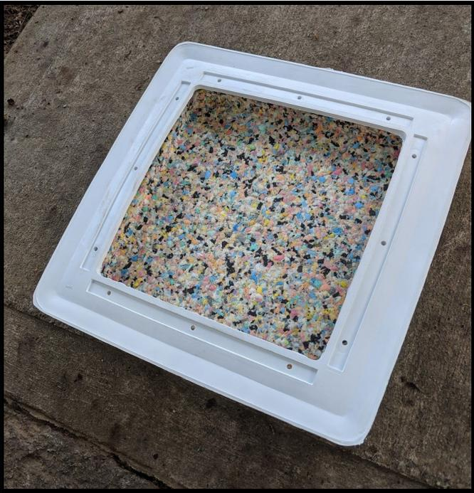
Decomposition of the Champion base. The metal stake is sunk into the ground which secures the base. The stake is easily removable with 2 bolts. These bolts will be undone and the connection from the base plate (top right) and the anchor (the stake) will go through the load-absorption system. Note the significant concavity of the base plate. Also note the foam within the base which provides some small load-mitigation (bottom left).
