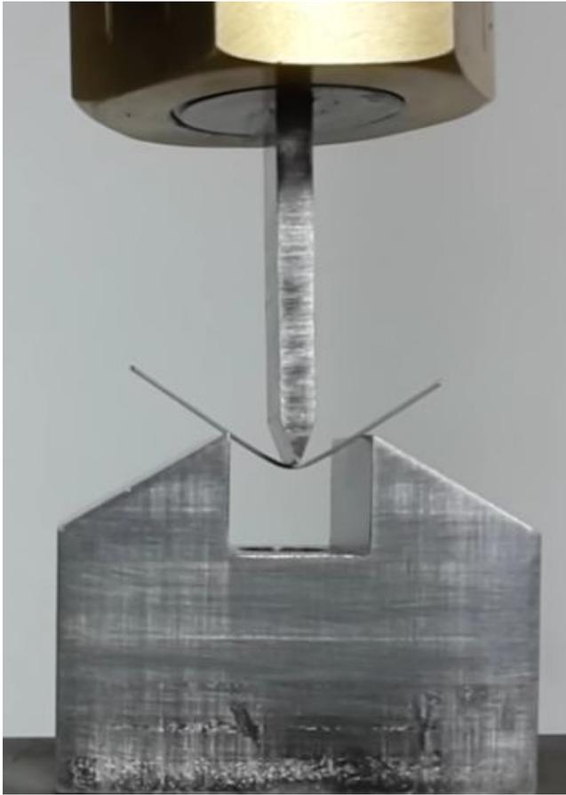
*Figure 3.3 (Left): Three-Point Bend test on a Nickel-Titanium Wire nearing maximum deflection*
