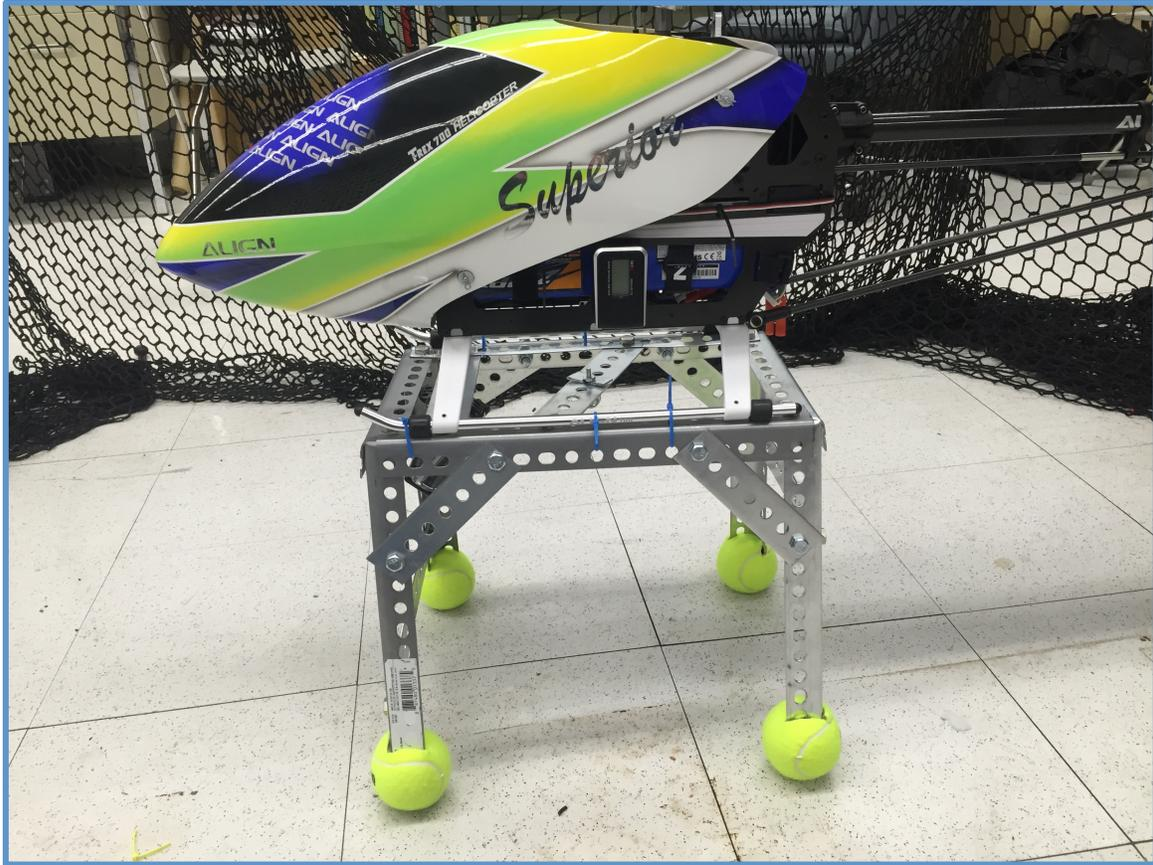
FIGURE 17: SIDE VIEW OF EXPERIMENTAL UNDERCARRIAGE ON T-REX 700
