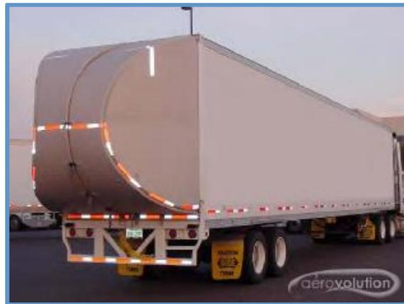
FIGURE 7: INFLATABLE BOAT-TAILING DEVICE [1]
