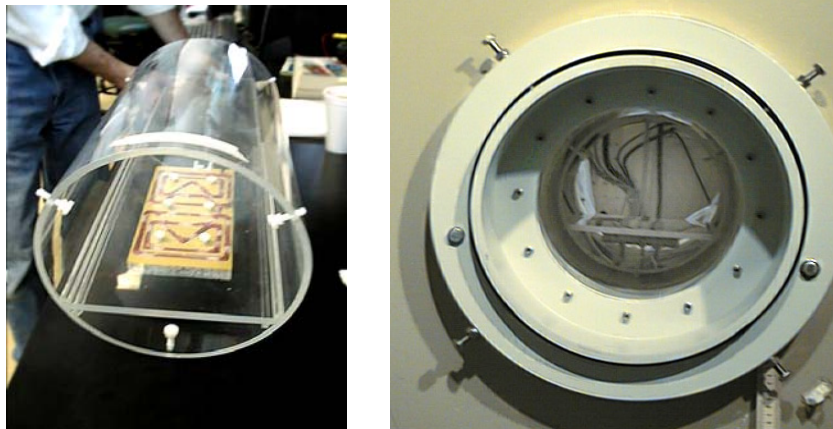
Figure 3.24: Photographs of the six-loop G_y coil placed in a 25 cm diameter Plexiglas tubular cylinder (left) and placed inside the 4.7T Bruker magnet with commercial gradient set (right).
