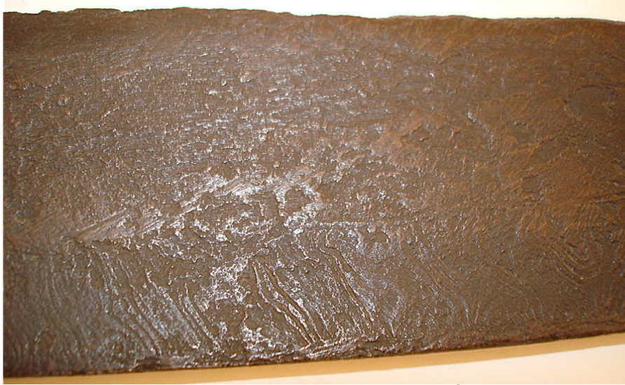
HAM 576, the blade of a sax sword from the 10 th century C.E., found in France. Note the lines that can be seen on the blade due to the pattern welding process.
