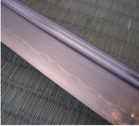
Figure 5: On this sword you can see the hamon. The round, bubbly pattern indicates a good hamon. The hamon is the pattern that forms when the edge is being hardened. ( www.wikipedia.com )
