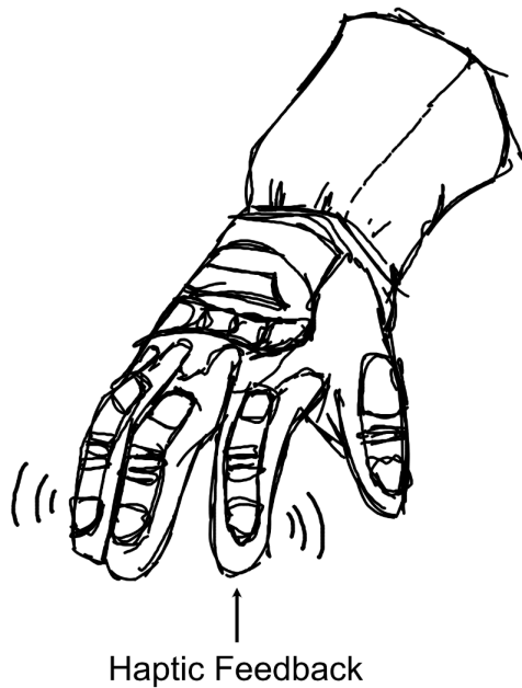
Figure 1: Welding glove and AR welding helmet. The glove is connected to an external sensor that is able to send signals to the glove for haptic feedback. The AR welding helmet has an AR screen, thermal camera in the front, and external buttons on the side.
