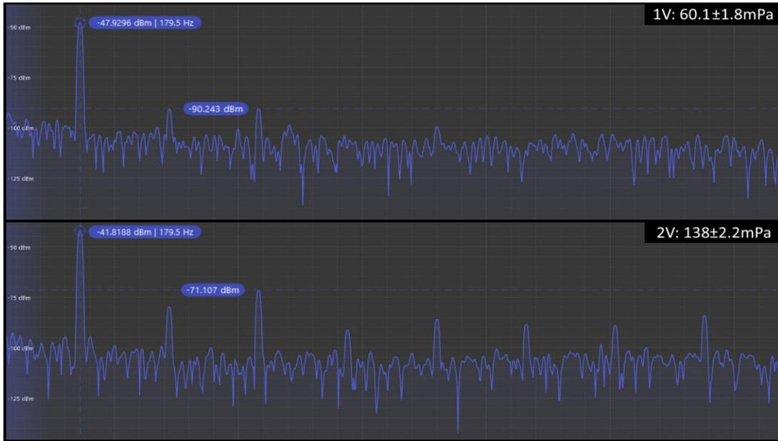
**Fig. 32** Speaker's frequency FFT at 180 Hz at 2V and 1 V with 18x averaging.
