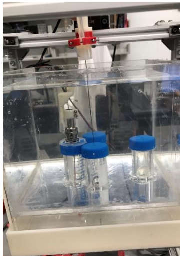
Figure 35. The USCT device imaging needle phantom.
