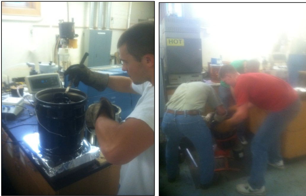
Figure 7: Left: Binder being added to aggregate; Right: Mixing the binder and aggregate
