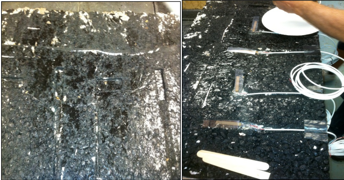
Figure 15: Left: Imprints in slab for strain gages; Right: Strain gages epoxied onto slab
