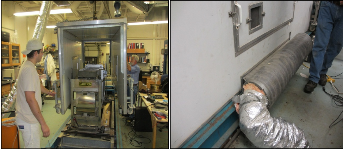
Figure 12: Left: Environmental Chamber being lowered over slab; Right: Heating vents
