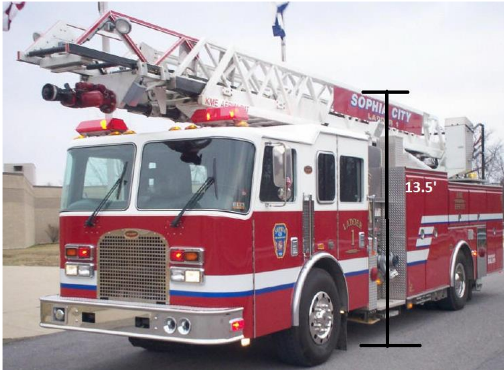
Figure 46: Fire Truck Height Dimension
