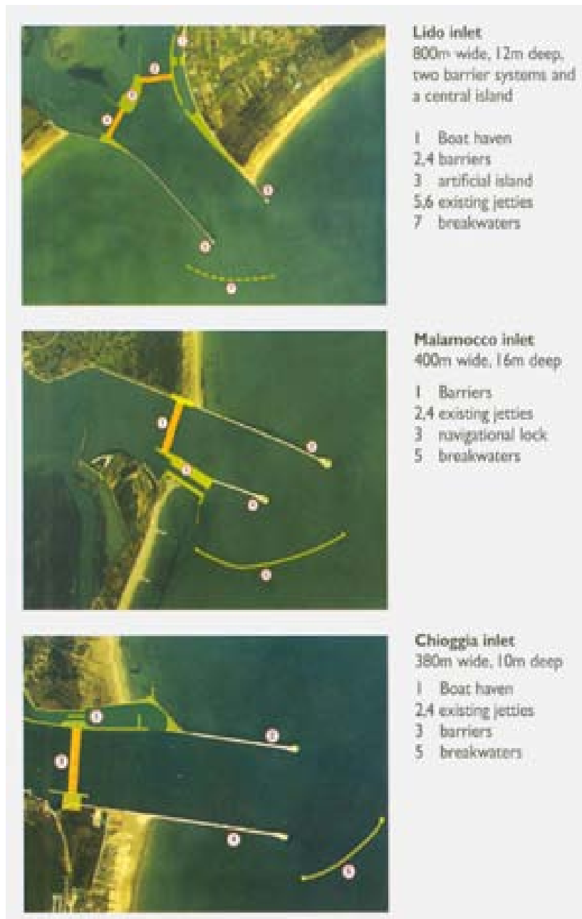
Figure 18: The proposed setup of the MOSE system at the three crucial inlets in Venice 63
