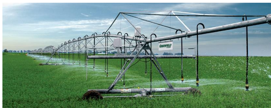
Figure 12: Lateral-sprinkler irrigation system
