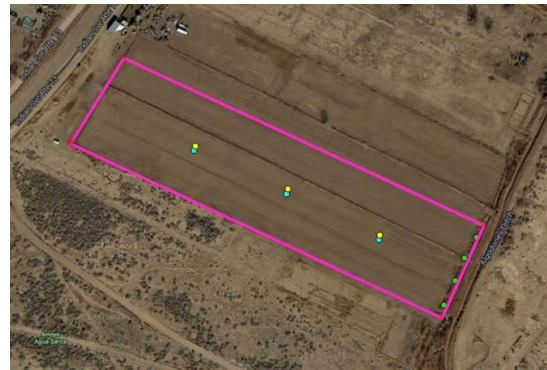
Figure 33: Field 29 with tensiometers installed. The yellow dots are the tensiometers that were placed 6 inches into the ground, while the blue dots are the tensiometers installed 12 inches deep. The green dots are bubblers.
