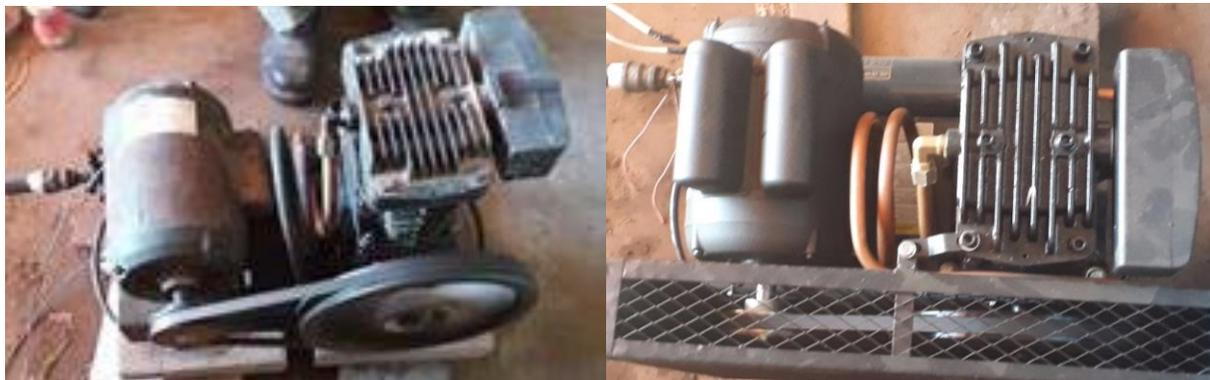
*Figure 4: Previous air compressor (left) and new air compressor (right)*
