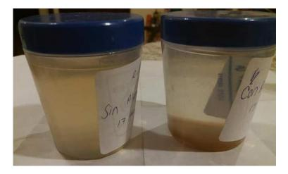
Figure 4: Water from Río Verde without aluminum sulfate (left) and with aluminum sulfate (right) after settling for less than 30 minutes.
