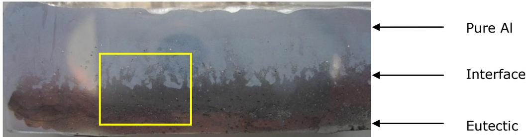
**Fig. 19: Developing striations across the interface. (The reflection in the background is the camera lens).**
