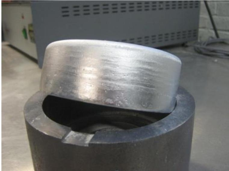
**Fig. 28: 206 Cast via CDS - No hot tearing.**
