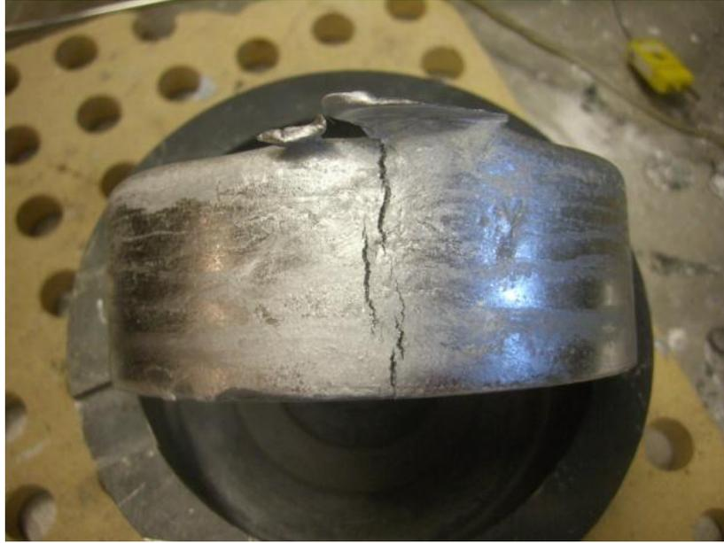
**Fig. 49: 2014 – Regularly cast – Moderate crack.**
