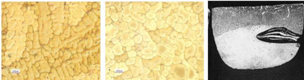
**Fig.13: From left to right a) Homogeneous liquid solidifying (dendritic microstructure) b) Reaction mixing, (globular) c) Quenching (severe segregation).**
