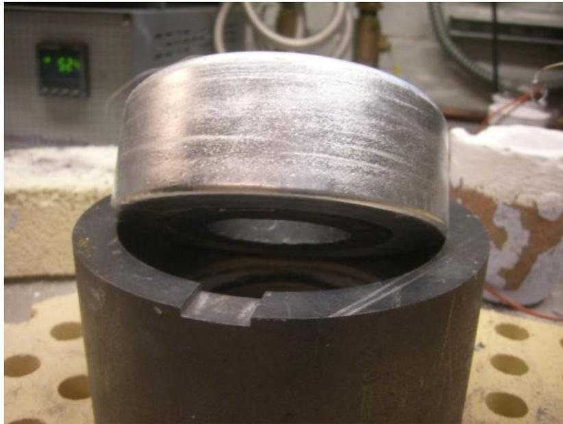
**Fig. 50: 2014 – Cast via CDS – No crack.**
