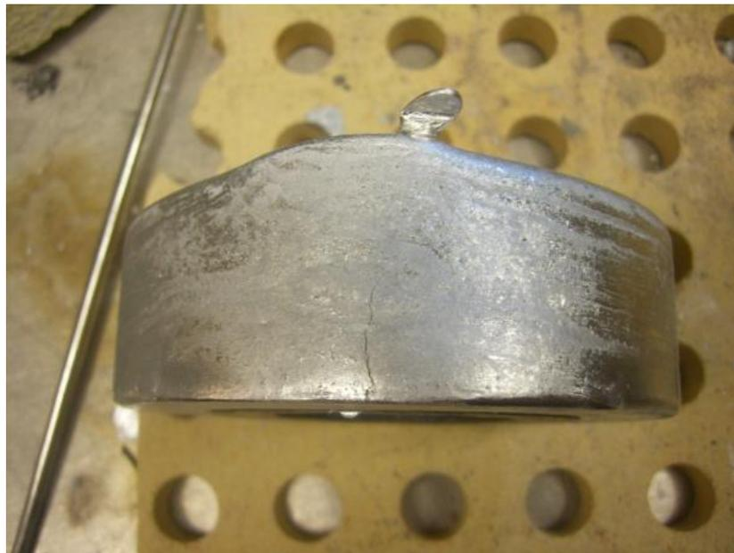
**Fig. 48: 2014 - Regularly cast - Hairline Hot Tear.**
