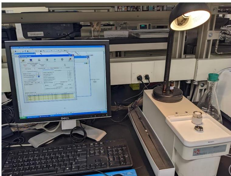
**Figure 6.** Differential Scanning Calorimeter as seen in the Gericke Lab. Original photo.
