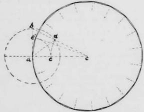
Draw ab perpendicular to ac at a and equal to one-half ac. Draw bc. With radius ab describe arc bd. With radius cd describe arc de, then ae = ae' is one side of inscribed nonadecagon very nearly.
