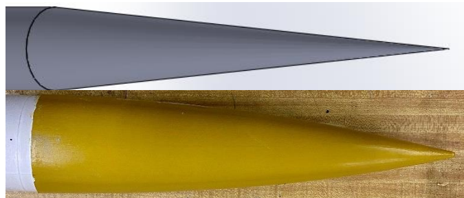
Figure 136: Comparison of the modeled nose cone (top) and the real nose cone (bottom)
