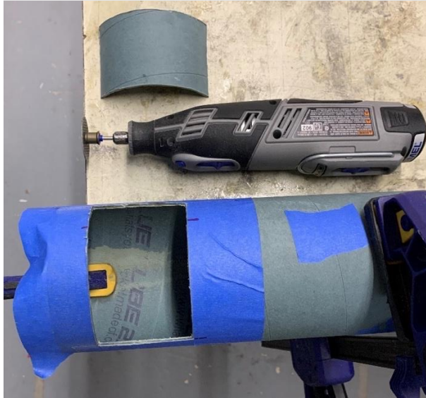
Figure 36: Airframe after the e-bay window was cut out
