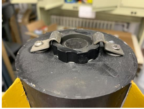
Figure 53: Motor retention system
