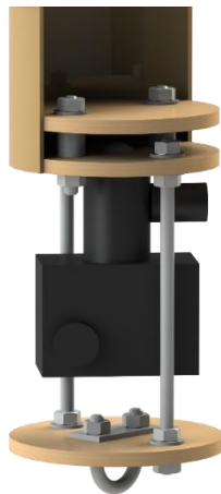
Figure 34: SOLIDWORKS model of the payload bay
