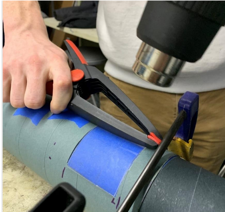
Figure 39: Molding process for the e-bay window
