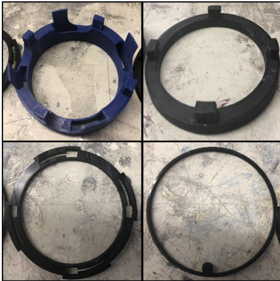
Figure 104: 3D printed parts for the gearing arrangement
