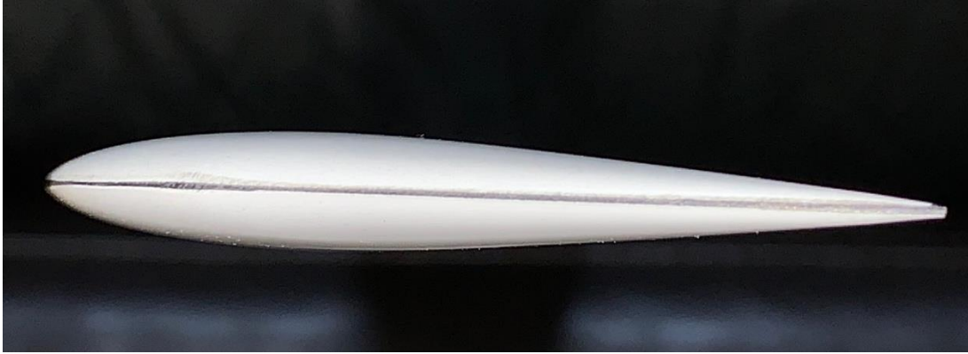
Figure 61: Photo showing the cross-section of the rotor blade
