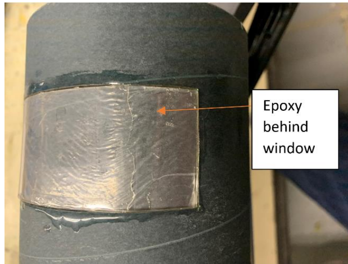
Figure 42: Epoxy seepage behind window
