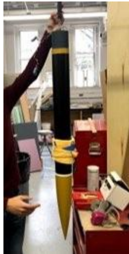
Figure 100: Rocket orientation during nose cone separation test without shear pins
