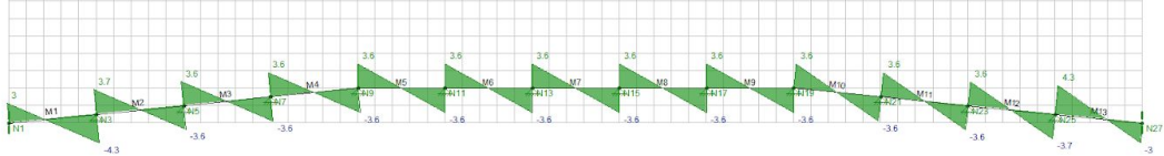
Figure B7: The resulting axial forces displayed graphically for the 1.2D + L + 0.5 S Load Combination.
