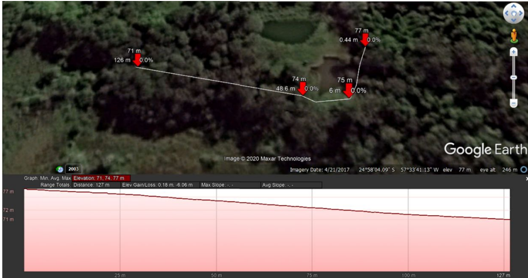
Figure 7: Outer Canal Elevation Profile
