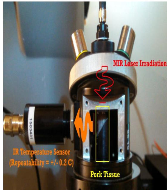
Figure 8: Microscope set up to test heating effect of 800nm & 980nm laser
