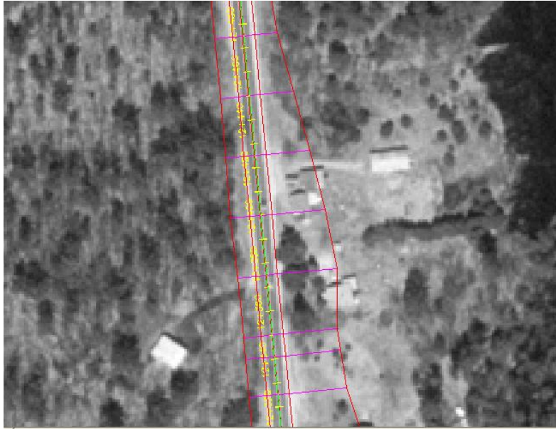
Figure 7-8. Impacts to Existing Residence STA 12+320 to 12+420.
