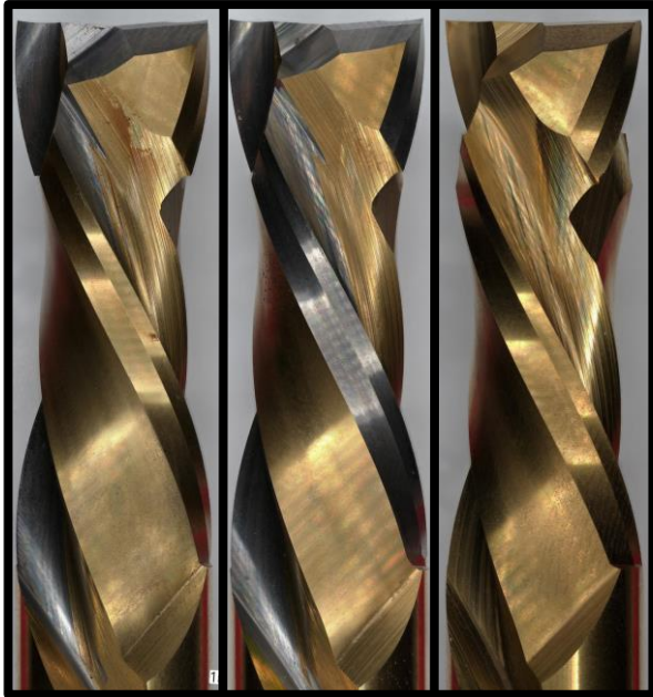
Figure 3: Left: flute grind, center: full geometry grind, right: brand new endmill.
