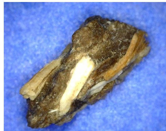
Figure 5: Sample of non-homogeneous fiberboard material.
