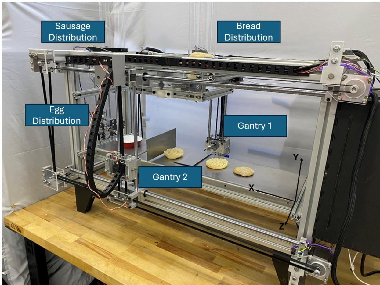
Figure 58: Full Breakfast Sandwich Robot Assembly
