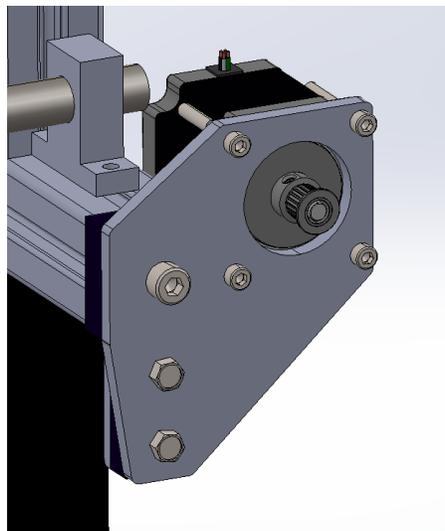
*Figure 20: NEMA 23 Motor Mount CAD Rendering*
