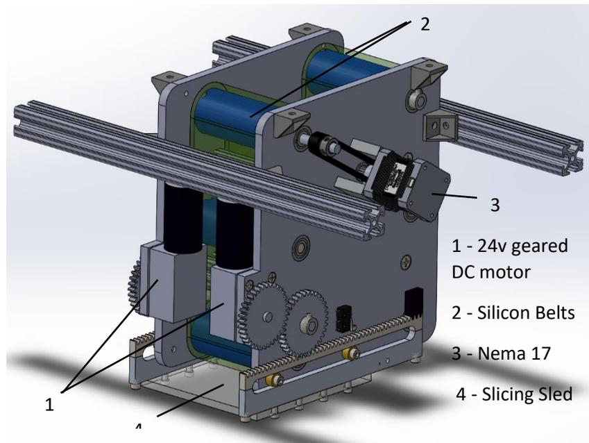
Figure 35: Cheese Distribution and Slicing System CAD render
