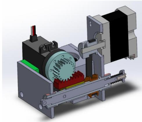
Figure 24: Utensil Change Locking Mechanism CAD Render
