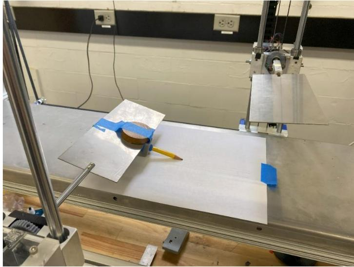
*Figure 82: Gantry Motion Testing in X Direction*
