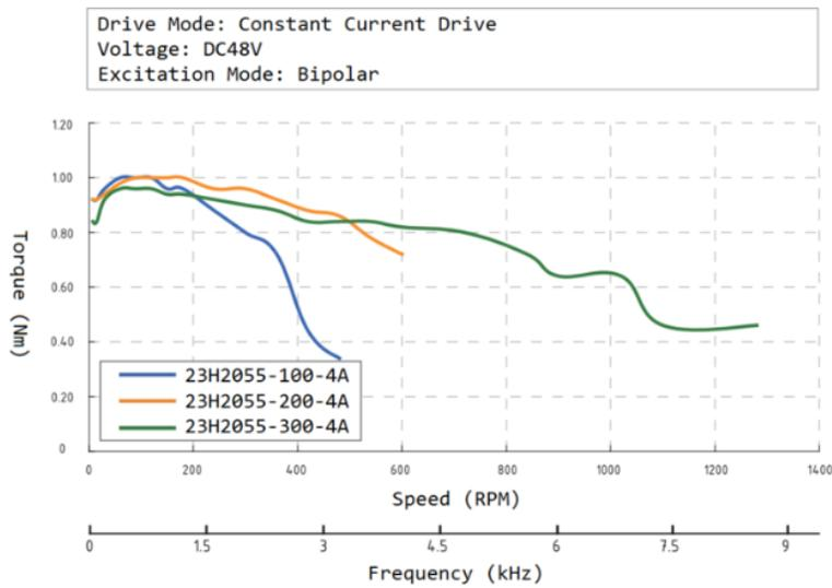
Figure 17: 2phase 2Amp 57mm NEMA 23 stepper motor torque-speed curve (NEMA 23 2phase 2Amp 57mm — DINGS' Motion USA)
