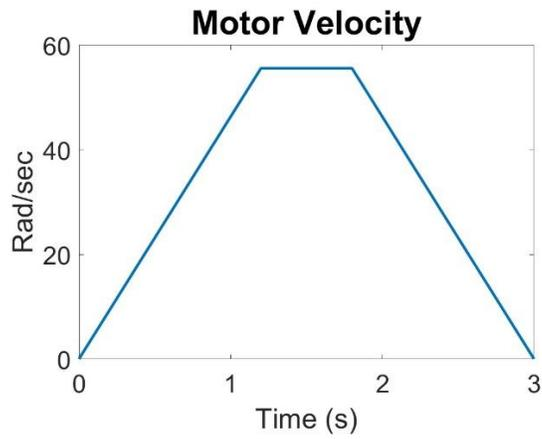
Figure 15: Required Individual Motor Velocity Output MATLAB Sim
