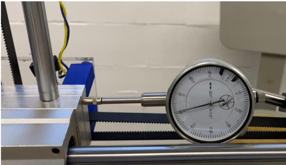
*Figure 83: Dial Indicator Test on X axis.*
