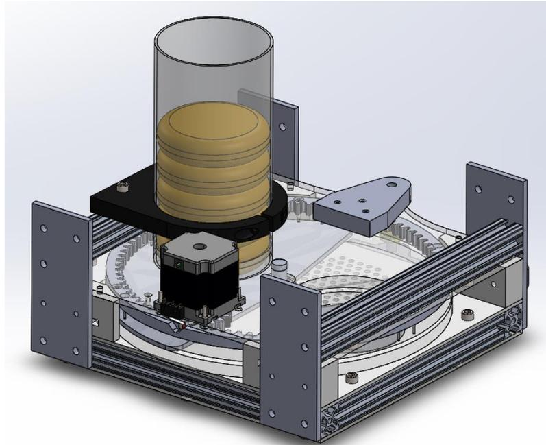
Figure 33: CAD model of bread distribution system.
