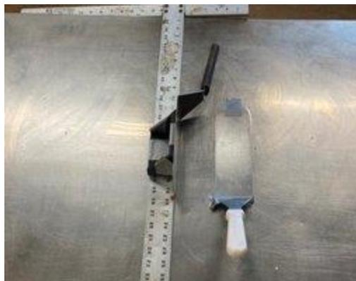
*Figure 4: Spatula Interaction with Food Test Set Up*
