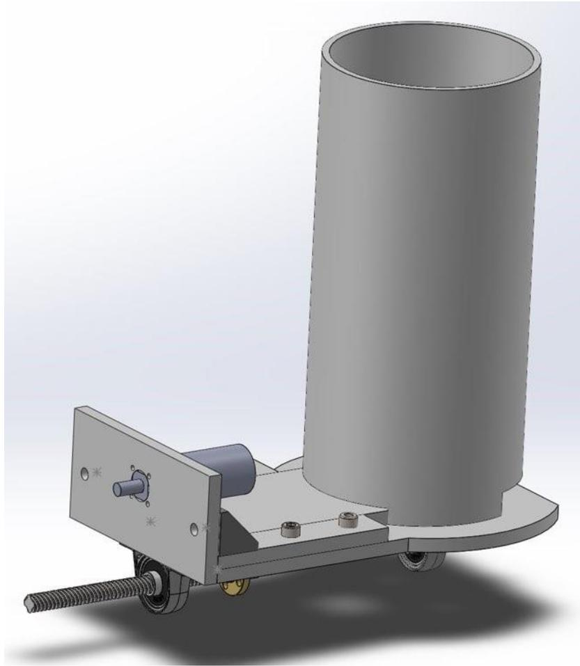
*Figure 45: CAD model for sausage distribution approach 1*
