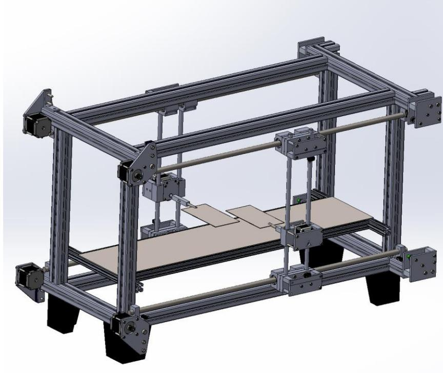
*Figure 19: CAD Rendering of Gantry Design*
