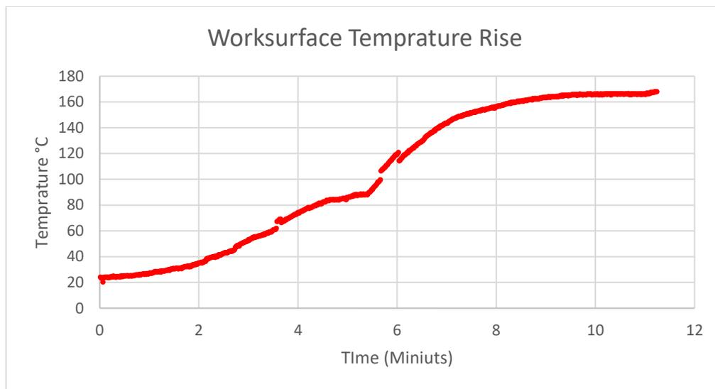
Figure 84: Worksurface Temperature Rise Over Time
