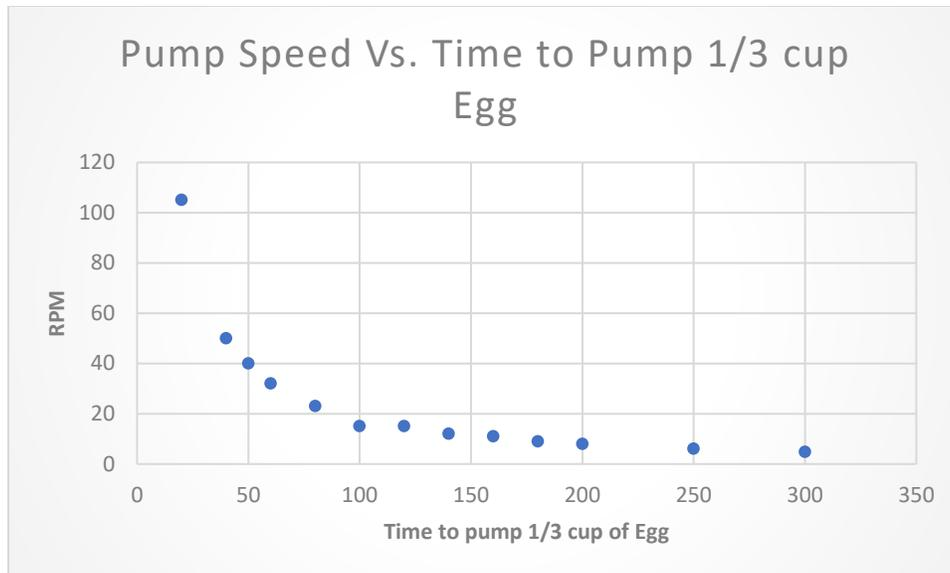
Figure 39: Graph of pump speed, in RPMs, versus the time it takes for the pump to transport 1/3 cup of liquid egg, in seconds.
