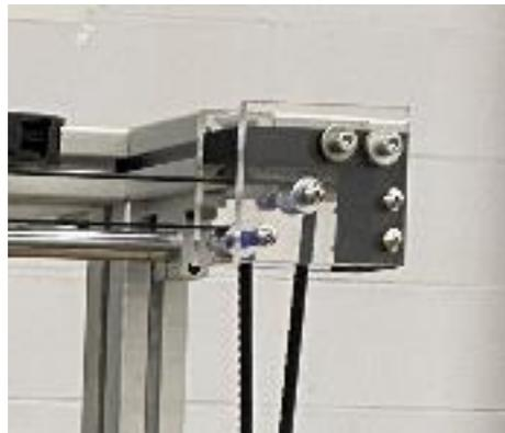
*Figure 62: Corner pulley bracket*
