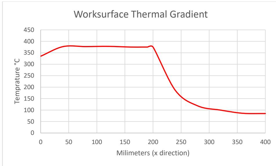
Figure 85: Worksurface Thermal Gradient
