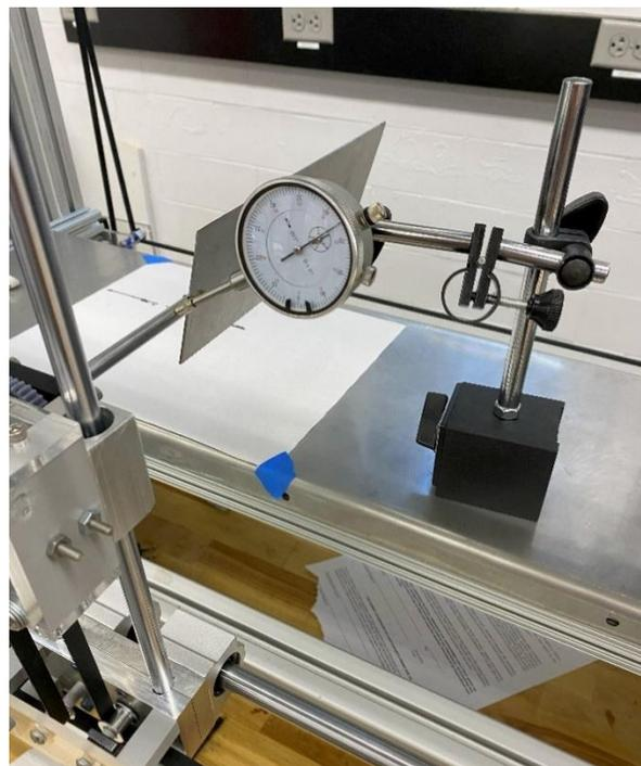
*Figure 67: Spatula Alignment and Trimming*
