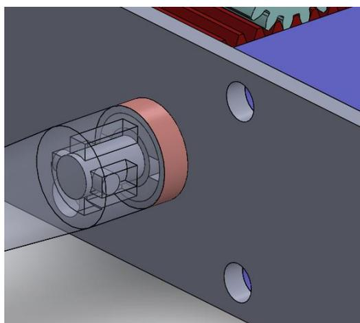
Figure 27: Utensil Change Locking Mechanism
