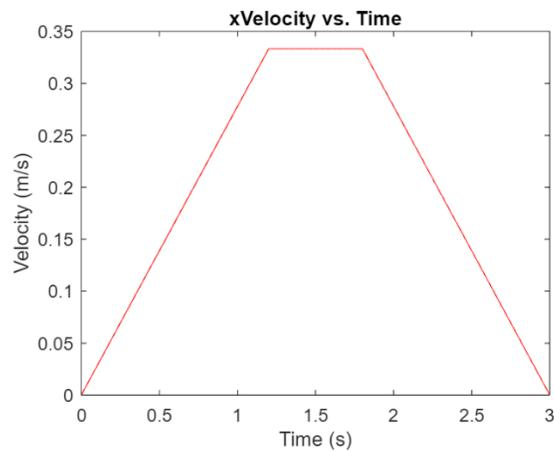
Figure 89: End Effector Velocity in X Direction
