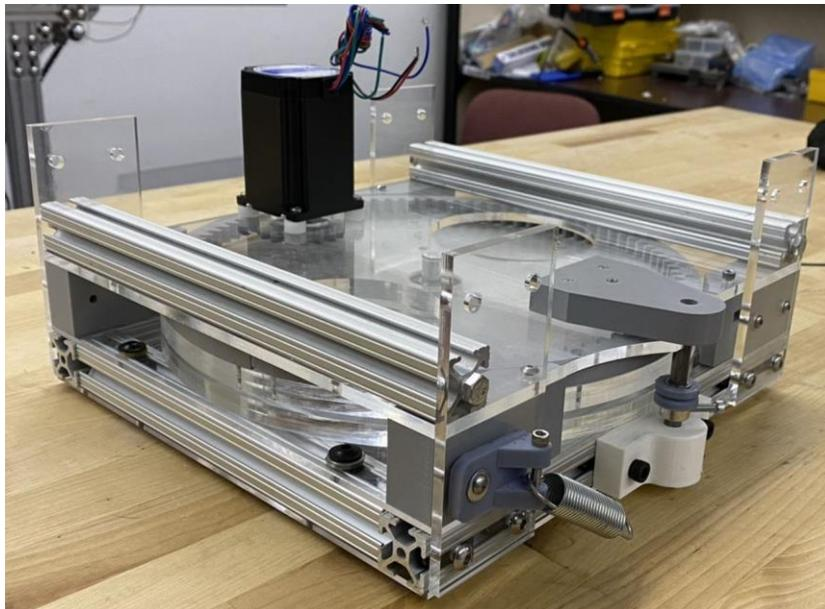
Figure 34: Finished bread distribution system.
