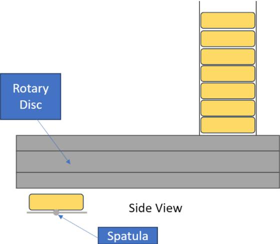
Figure 32: Side View Diagram of bread distribution system.
