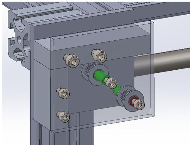
*Figure 21: Corner Pulley Brackets CAD Rendering*
