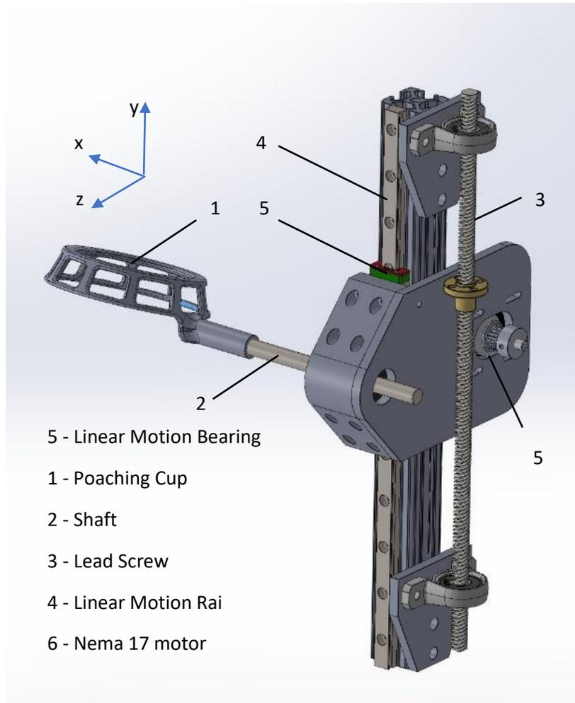
Figure 41: Egg Cooking Apparatus Approach One
