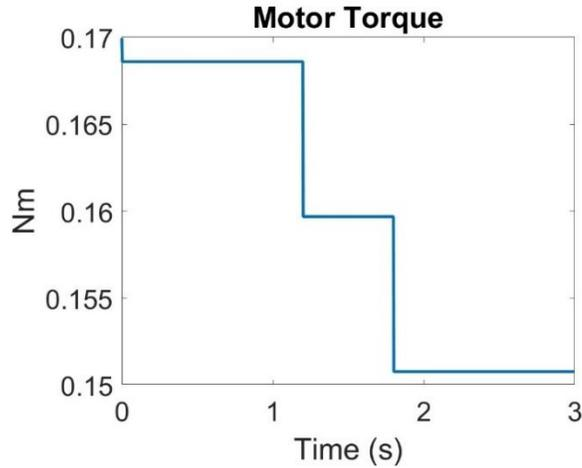
Figure 16: Required Individual Motor Torque Output MATLAB Sim
