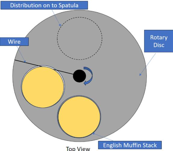
Figure 31: Top View Diagram of bread distribution system.
