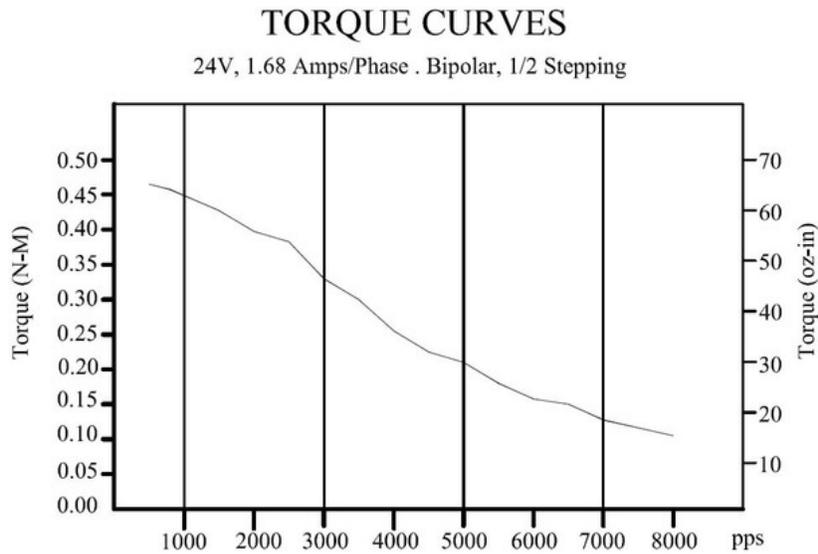
Figure 42: NEMA 17 Torque - Speed Curve (open builds part store)
