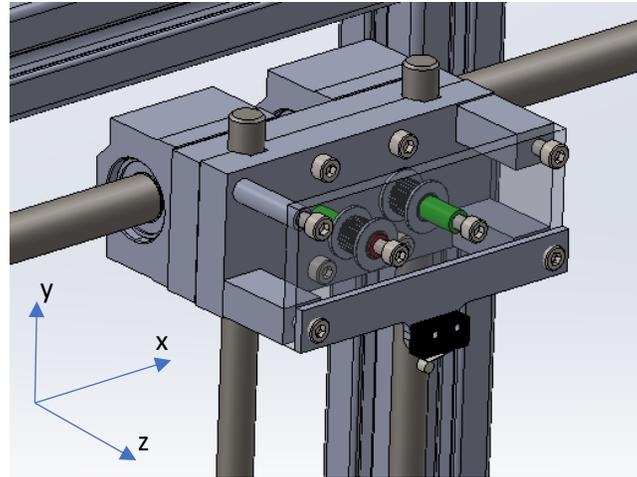
Figure 22: Y Axis Alignment Mounts CAD Rendering
