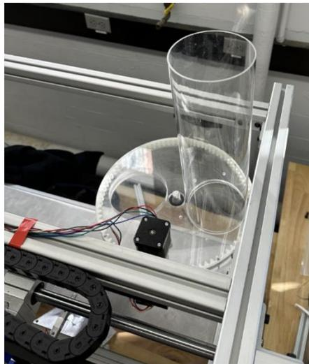
Figure 48: Sausage Distribution System installed on the robot
