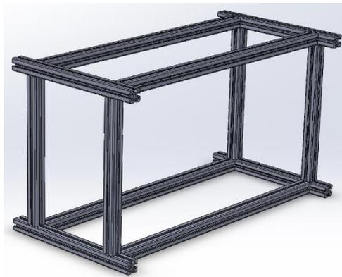
*Figure 18: Robot Frame From 8020 Extrusion*
