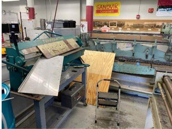
*Figure 72: Work Surface Bending Operation*
