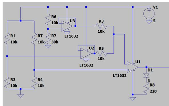
Figure 53: Oven Fail Safe Circuit Design
