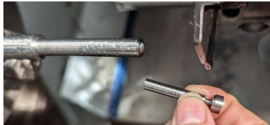
Figure 15: Broken Shaft 2 in the Lathe
