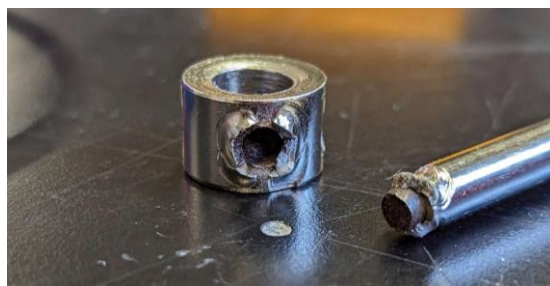
Figure 21: Broken Hand Crank Generator Handle
