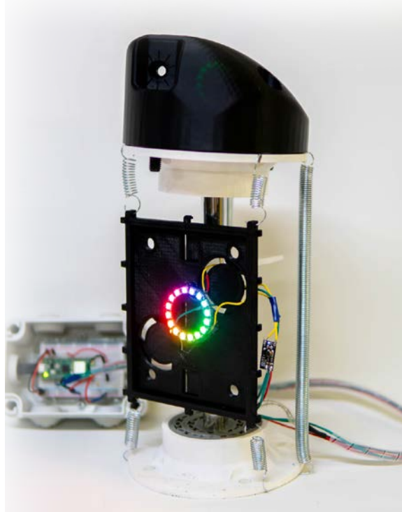
Figure 16: Model with hit window removed to expose ring light that is controlled by software
