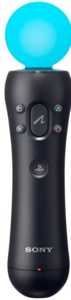
Figure 4: PlayStation Move controller with motion tracked ball on end
