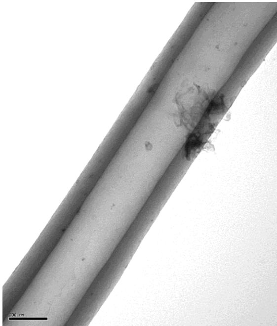
Figure 7: TEM image of avidin-glucose oxidase nanotube (scale bar represents 100 nm)
