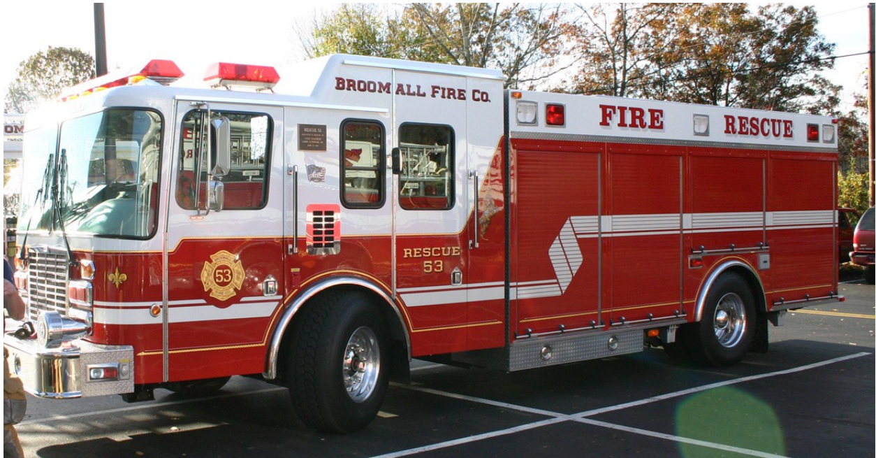
Figure 5 Broomall Rescue 53, example of a rescue apparatus without pump or tank
