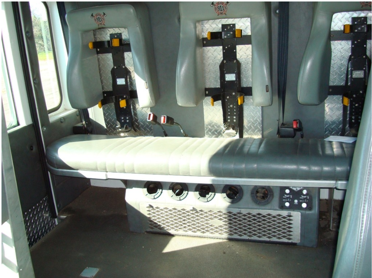
Figure 8 Typical seat-mounted SCBA brackets 33
