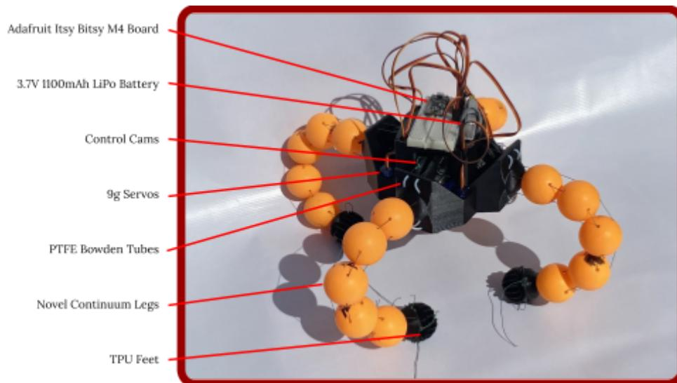
Figure 8: An image of the full SUSA CROQ implementation. On the left, labels describing the components of the robot.
