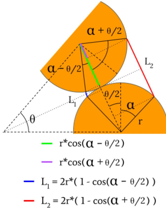
Figure 2: An illustration showing the string lengths on either side of the actuator, given a bending angle  $\alpha$ .
