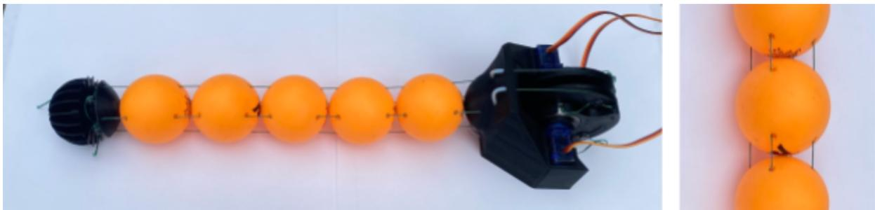
Figure 1: An image showing a SUSA module. On the right, a closeup of the actuation cables feeding through the actuator.
