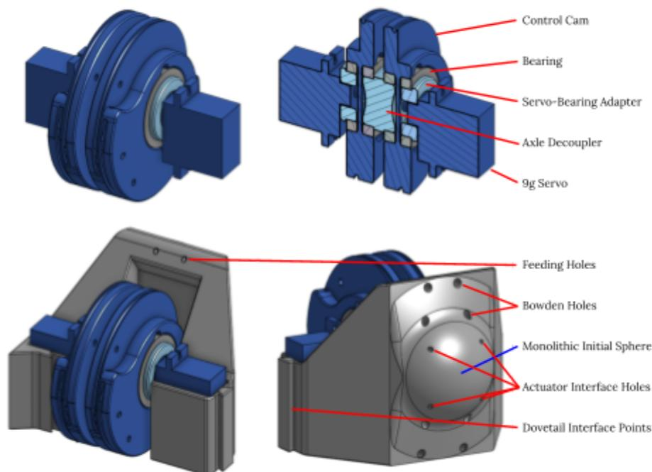
Figure 9: A diagram of the full SUSA module, omitting actuator spheres. Important, functional features are labeled. Top: Coaxial servo assembly, Bottom: Full module (omitting actuator spheres)
