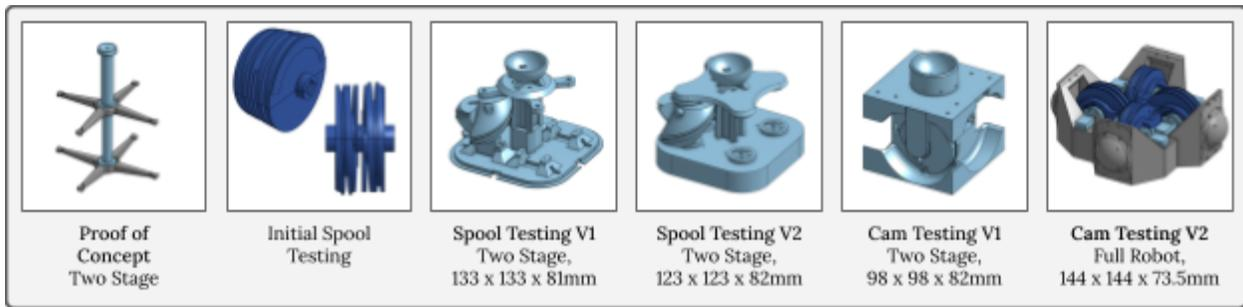
Figure 6: A diagram of each milestone version of the SUSa actuator. The differences between each version are discussed in the Mechanical Development section.
