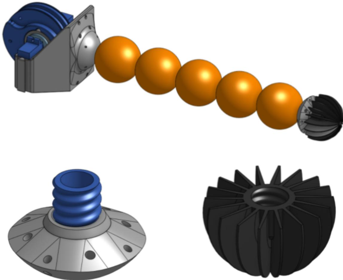
Figure 10: A CAD image of a full SUSA module. On the top, the full module including the actuator spheres and end effector with flexible foot. In the bottom left, a closeup of the partial sphere with machine screw holes, cable holes, and central screw interface. The partial sphere has a female screw interface for printability, with the male screw being printed separately. In the bottom right, a closeup of the finned, TPU foot. The thin (0.6mm) fins allow easy deformation around features.
