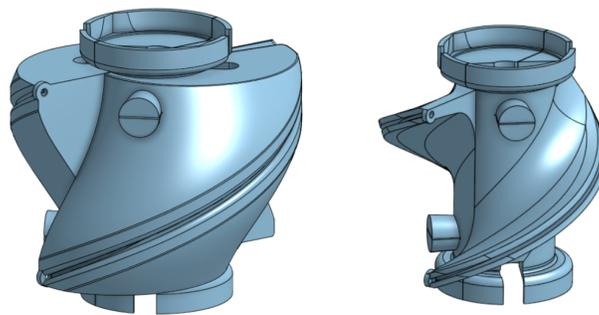
Figure 7: A comparison between the helical spool with the original cable guide and modified cable guide. The modified cable guide follows the spooling surface at a constant offset of 3.5mm, whereas the original guide had an offset of up to 18mm.
