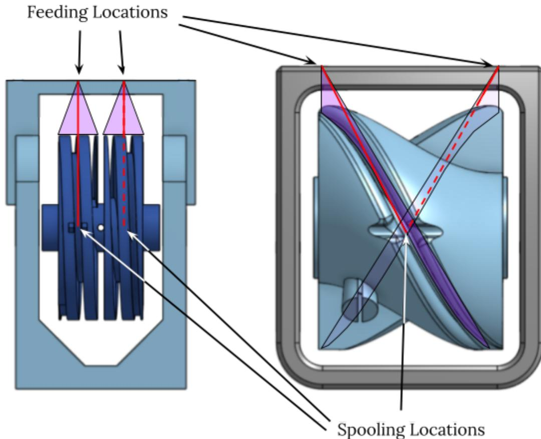
Figure 5: Feeding and spooling location of the first (left) and second (right) versions. Initial cable location is marked in red, with the range in spooling points highlighted in purple. Feeding location is defined as the point to which the cable feeds from the spool to the actuator. Spooling location is defined as the point at which the cable interfaces with the spool surface.
