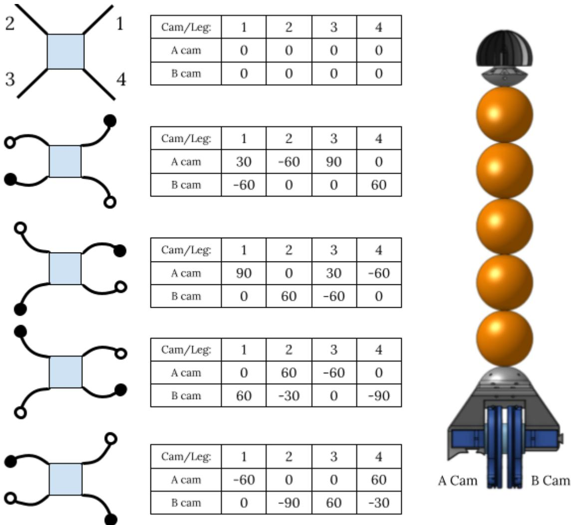
Figure 11: A diagram showing the four positions the robot takes when completing a walking gait (far left). Each leg is depicted as a curve with a circle on the end. A filled in circle denotes a foot touching the ground, while an empty circle denotes a lifted foot. On the right, a top view of the SUSA that labels the A and B cam, whose positions (degrees displaced from neutral position) are shown in a table for each walking position.
