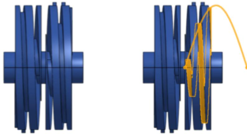
Figure 4: A side view of the initial version of the spool of varying radius. On the right, the spooling surface and sinusoidal curve is highlighted. As the cable is wound, it is pushed across the width of the spool by the cable guides.
