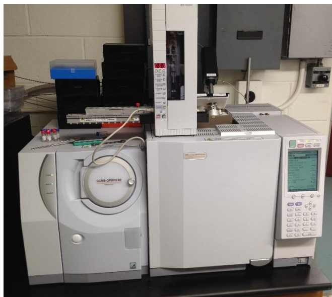
Figure 8: Gas Chromatograph Equipment Used for Continuous and Batch Analysis
