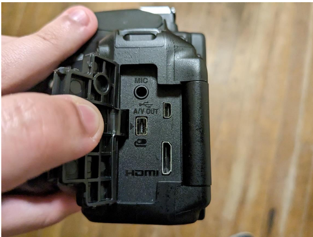
Figure 3.3. Available ports on the D5300, which include Mic Out, A/V Port, and HDMI.
