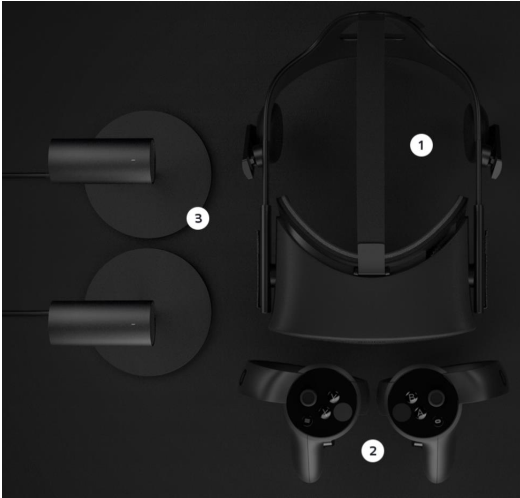
[Figure 27: Oculus Rift, 1. Headset, 2. Touch controllers, 3. Sensors. (Oculus Rift, 2018)]
