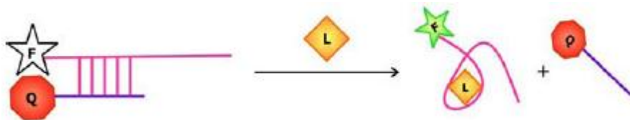
Figure 4. Change Induced in a Structure-Switching Aptamer upon Binding to its Target Molecule (Mok et al.)
