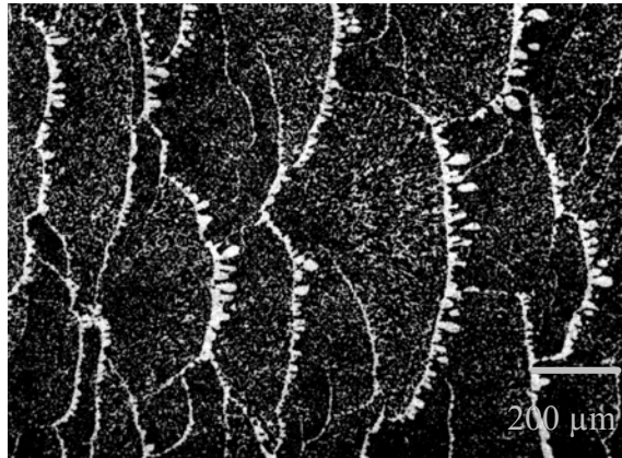
Figure 19: Overmodification bands in aluminum silicon eutectic sample. Sample obtained by directional solidification experiments at a growth rate of 120 mm/h. Thick bands with dendrites and thin bands can be observed [30]
