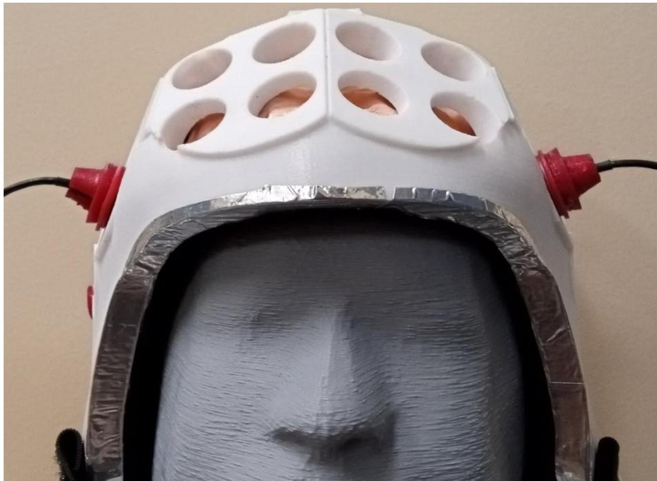
*Fig. 19. Microwave imaging helmet with positions for multiple small antennas, fitted to a plastic head mock-up. Only two of the positions are populated with antennas in the figure.*
