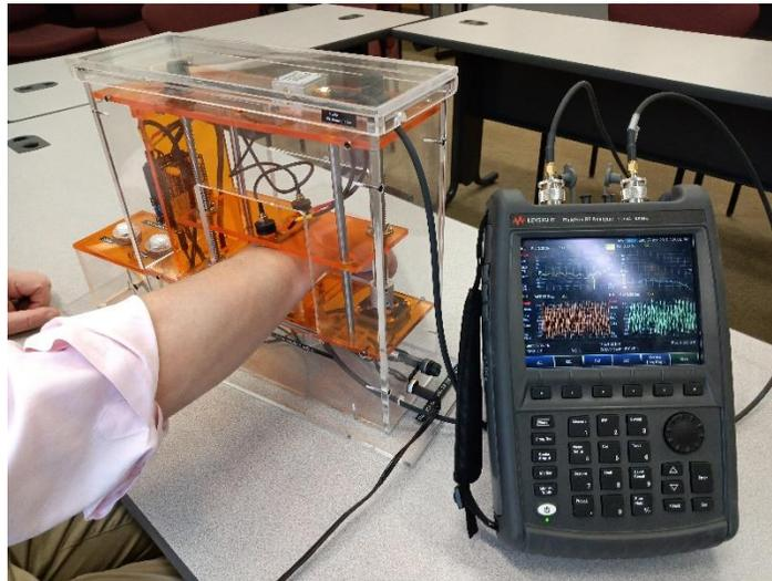
*Fig. 9. Experimental setup connected to portable Keysight FieldFox N9914A network analyzer and performing measurements. Measurements of reflection and transmission coefficients  $S_{11}(f)$ ,  $S_{21}(f)$  as functions of frequency are performed in less than 0.5 seconds. The device top is then raised to its original position (3-7 sec). [6]*
