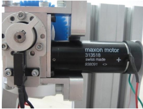
Figure 16: Maxon motor on 2-DOF joint
