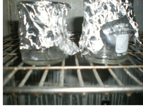
Figure 4 - Thermal Crosslinking of Polymer Solution in Washburn Labs
