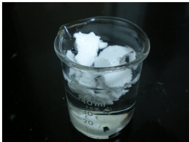
Figure 16 - Dissolving Styrofoam(Polystyrene) in acetone
