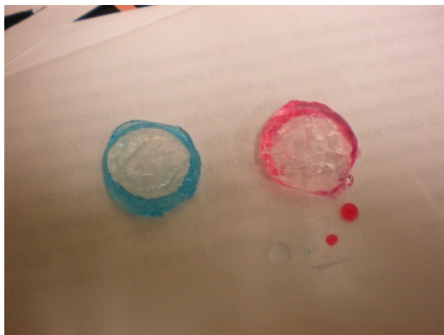
Figure 17 - PAA/PVA samples after coatings applied
