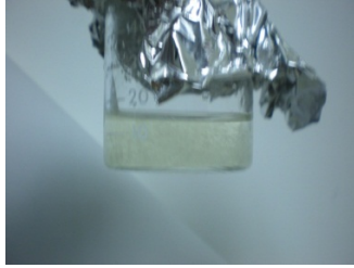
Figure 1 – NIPAM Polymer Solution in initial stages of Crosslinking
