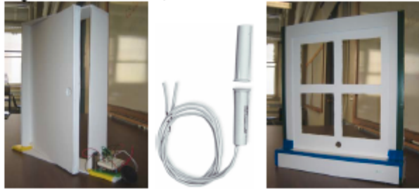
Figure 5: Window Prototype (left), Magnetic Switch Used (center), Window Prototype (right)
