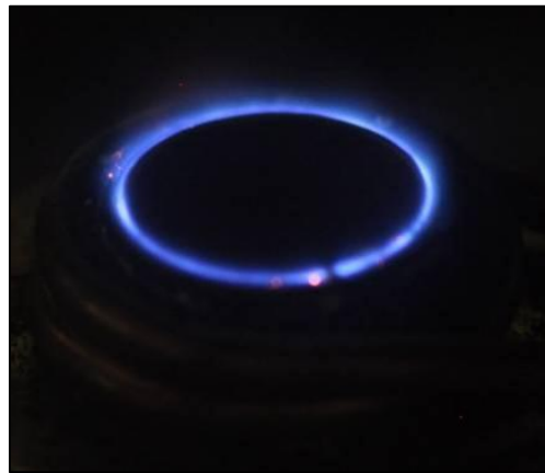
Figure 2.5: Premixed methane-oxygen pilot flame.
