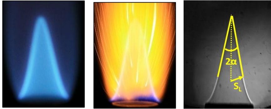
Figure 3.2: Flame images, a) Direct image of gaseous premixed flame; b) Direct image of gas-dust premixed flame; c) Shadowgraph image of gas-dust premixed flame.
