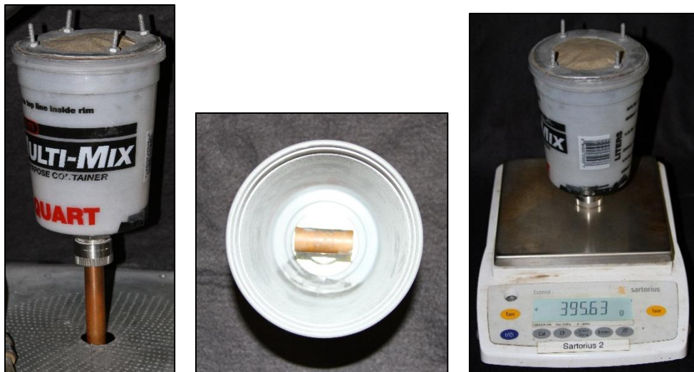
Figure 2.13: Dust hopper for dust calibration.
