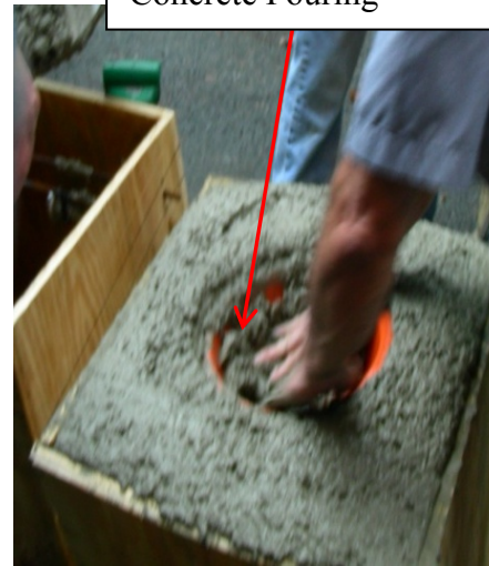
Figure 13 Bowl Placement in Concrete Block
