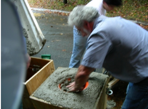
Figure 16 Construction Sequence for the Creation of the Pothole
