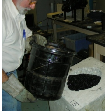
Figure 16 Construction Sequence for the Creation of the Pothole
