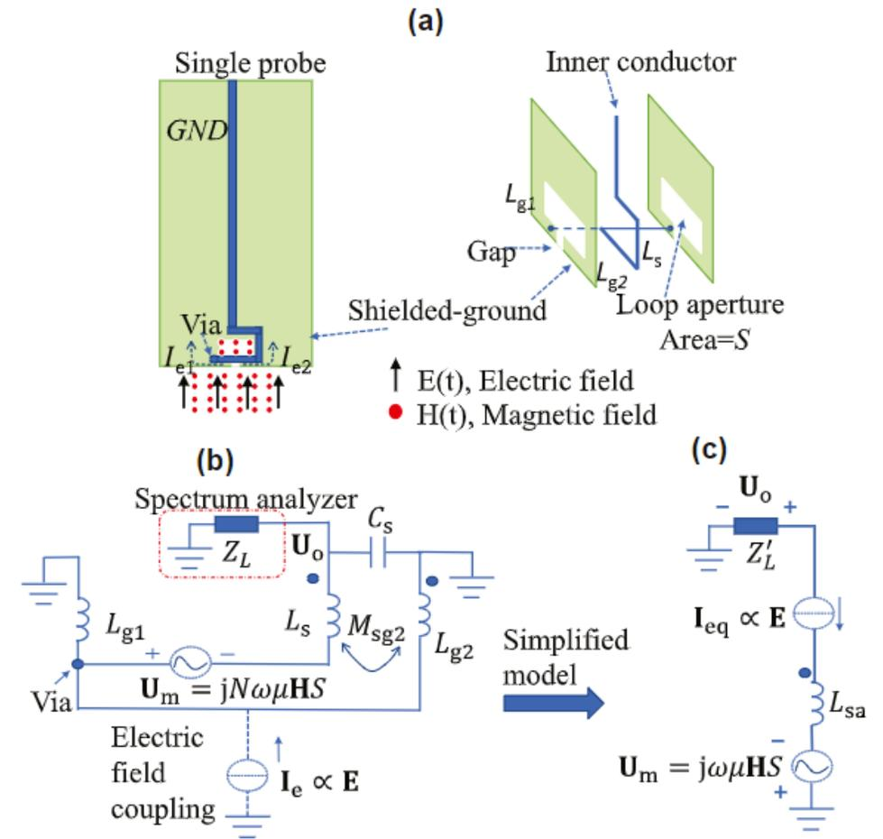
A popular single-shielded-loop magnetic field probe (a), its circuit mode (b) and simplified mode (c)
