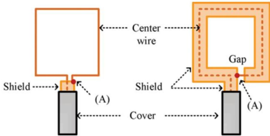
Square loop from a coax cable unshielded (left) and shielded (right)
