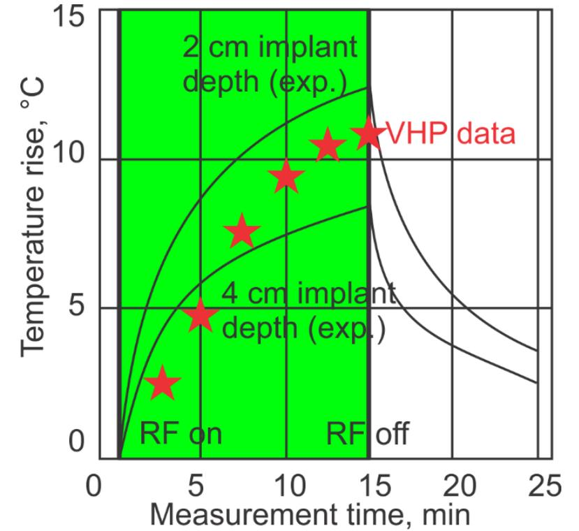
VHP results in relative agreement – differences attributed to variation in rod depth (vs constant depth of phantom) and changes in material properties
