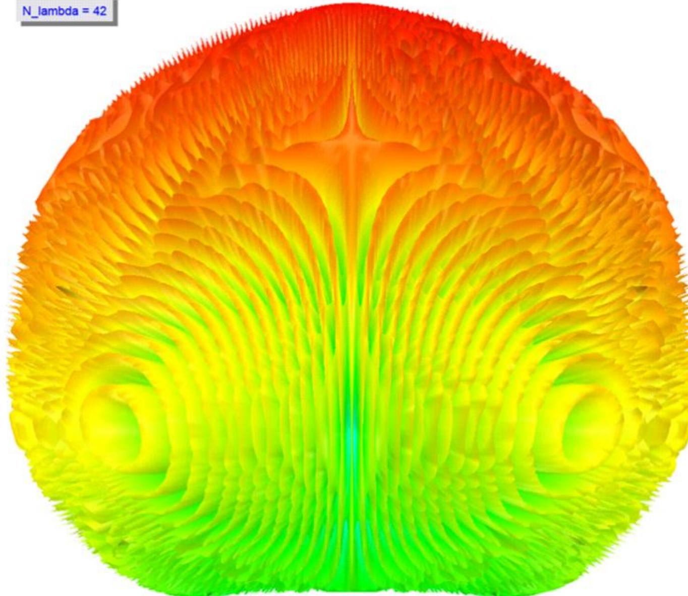
*Animation: Combined Far-Field Pattern of Two Antennas vs. Antenna Spacing; Made w/ Ansys HFSS SBR+*
