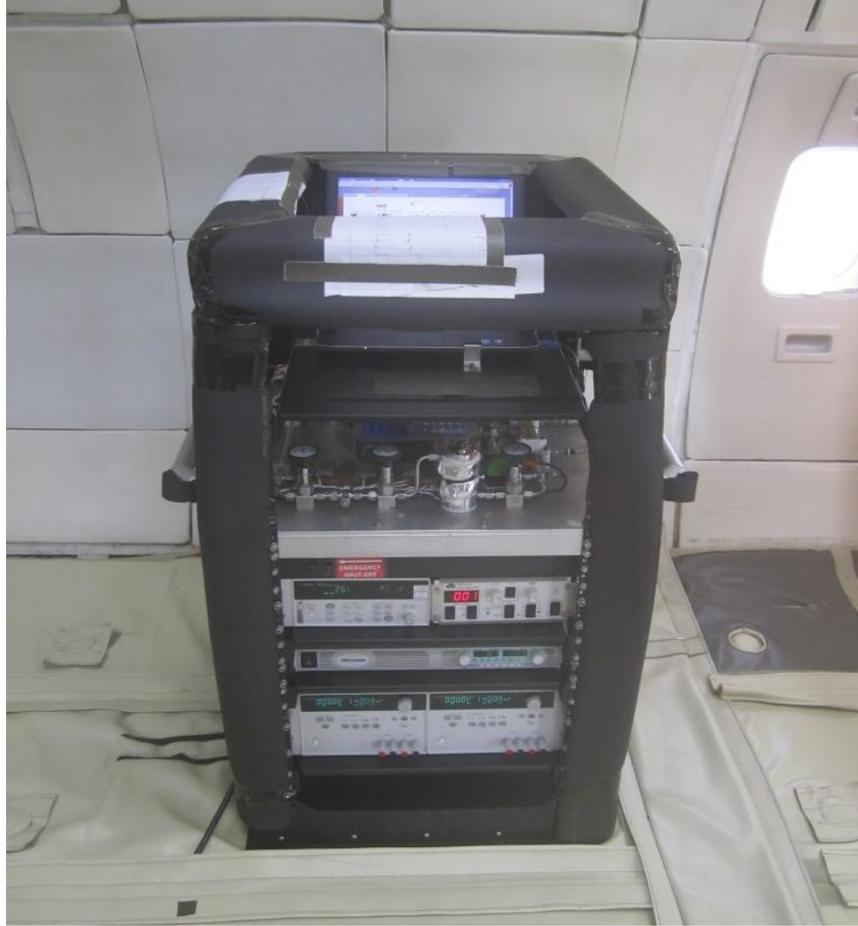
Figure 40: Vertical equipment rack installed in aircraft for micro-gravity tests
