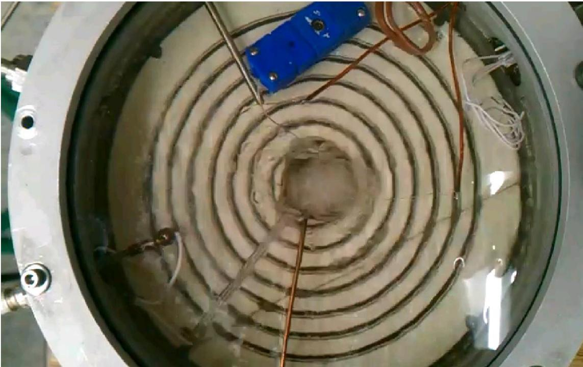
Figure 75: Image of pool boiling with pool depth: 10.0 mm, Heat flux:  $12.0 \text{ W/cm}^2$ , Applied EHD potential: 0 kV, Applied DEP potential: 2.5 kV
