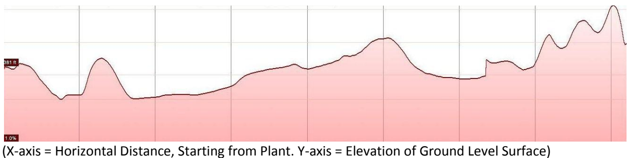
Figure 19. Elevation Profile under Site 9 Conveyor
