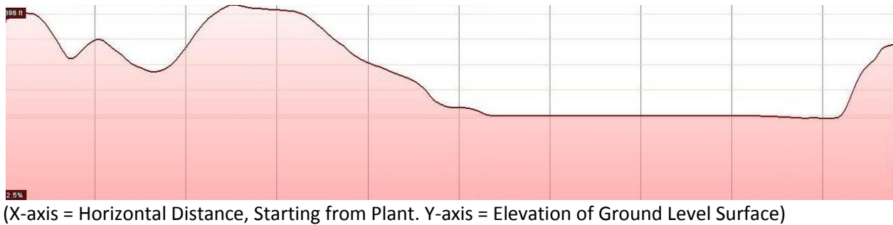
Figure 15. Elevation Profile under Plant Section Conveyor
