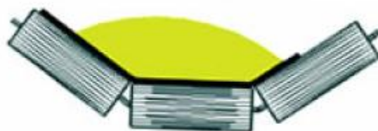
Figure 2. Belt Slippage on Idlers (Alspaugh M. , 2004)
